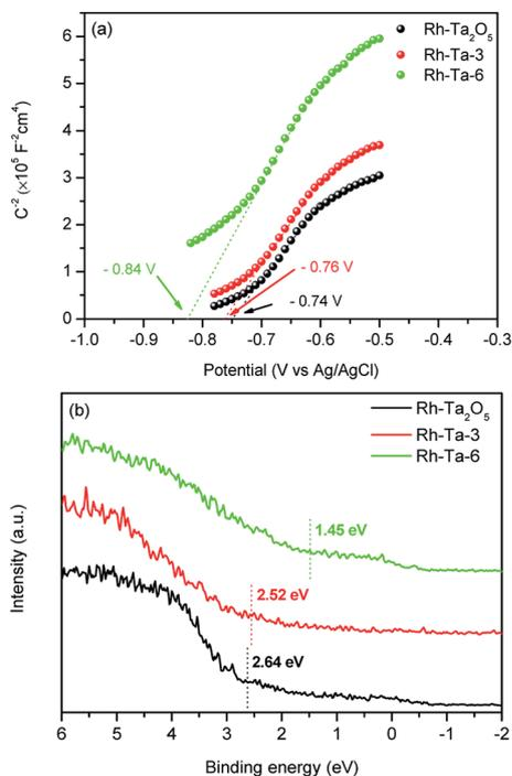
Fig. 8 (a) Mott-Schottky plots and (b) VB-XPS spectra of Rh-Ta<sub>2</sub>O<sub>5</sub>, Rh-Ta-3, and Rh-Ta-6 samples.
