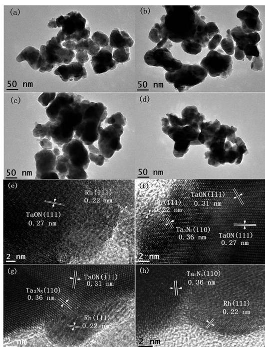
Fig. 2 TEM images of Rh-Ta-3 (a), Rh-Ta-6 (b), Rh-Ta-9 (c), Rh-Ta-12 (d) and HR-TEM images of Rh-Ta-3 (e), Rh-Ta-6 (f), Rh-Ta-9 (g), and Rh-Ta-12 (h).
