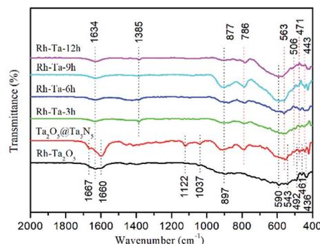
Fig. 5 FTIR spectra of Rh-Ta<sub>2</sub>O<sub>5</sub>, Ta<sub>2</sub>O<sub>5</sub>@Ta<sub>3</sub>N<sub>5</sub>, Rh-Ta-3, Rh-Ta-6, Rh-Ta-9, and Rh-Ta-12.
