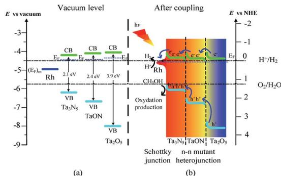
Scheme 2 Schematic illustration of (a) band positions of Rh, Ta<sub>3</sub>N<sub>5</sub>, TaON, and Ta<sub>2</sub>O<sub>5</sub> in vacuum level, (b) directional transfer of charge carriers in Rh-Ta<sub>6</sub> sample for Rh-Ta-6.
