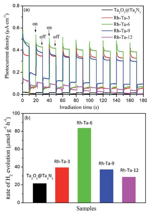
Fig. 7 (a) Photocurrent action spectra and (b) photocatalytic H<sub>2</sub>-evolution activities of Ta<sub>2</sub>O<sub>5</sub>@Ta<sub>3</sub>N<sub>5</sub>, Rh-Ta-3, Rh-Ta-6, Rh-Ta-9, and Rh-Ta-12.
