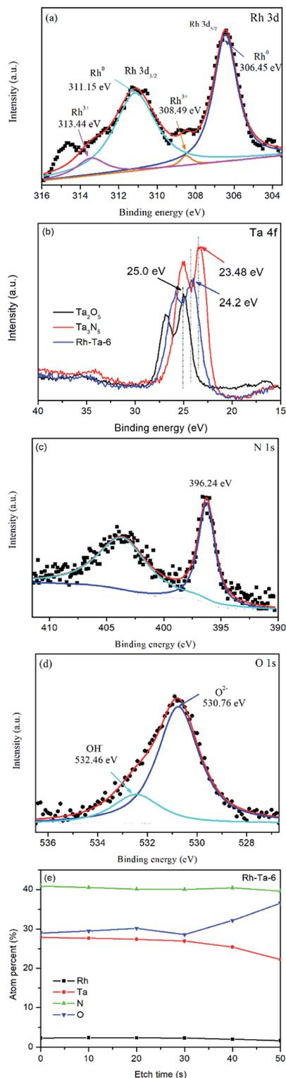
Fig. 4 (a) XPS spectra of Rh 3d for Rh-Ta-6; (b) XPS spectra of Ta 4f for Ta<sub>2</sub>O<sub>5</sub>, Rh-Ta-6, and Ta<sub>3</sub>N<sub>5</sub>; (c) high resolution XPS spectra of N 1s (d) and O 1s (e) for Rh-Ta-6; the atomic percentages of the etched layers for Rh-Ta-6 changing with Ar ion etching time.
