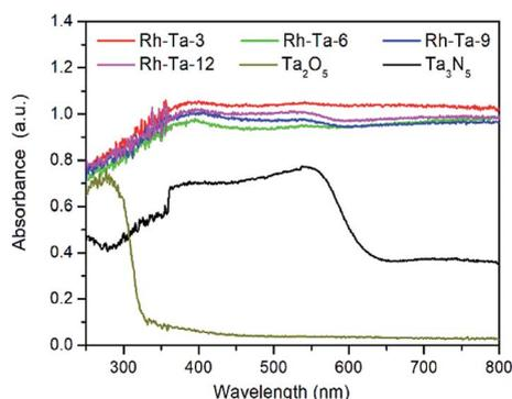
Fig. 6 UV-vis absorption spectra of Ta<sub>2</sub>O<sub>5</sub>, Rh-Ta-3, Rh-Ta-6, Rh-Ta-9, Rh-Ta-12, and Ta<sub>3</sub>N<sub>5</sub>.
