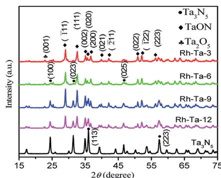
Fig. 1 X-ray diffraction patterns of Rh-Ta-3, Rh-Ta-6, Rh-Ta-9, Rh-Ta-12, and Ta<sub>3</sub>N<sub>5</sub>.
