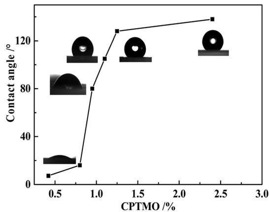
Fig. 6 Contact angle at different amounts of CPTMO.
