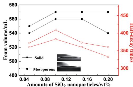
Fig. 9 Foam performance at different concentrations of SiO<sub>2</sub> nanoparticles.
