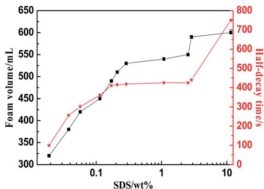
Fig. 8 Foam performance of SDS solutions at different concentrations.
