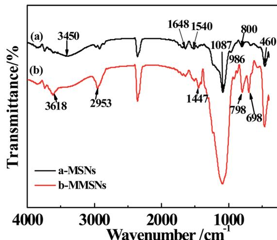
Fig. 7 FTIR spectra for (a) MSNs, (b) MMSNs.
