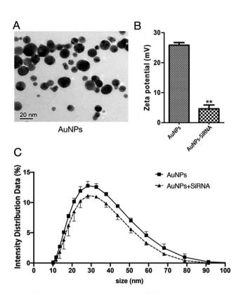
Fig. 3 Synthesis of AuNPs-siRNA $_{NPRI}$ . (A) Transmission Electron Microscope (TEM) images of bare AuNPs. Bars = 20 nm. (B) Zeta potential of the AuNPs (left) and siRNA-AuNPs (right). Student's t-test (\*, p < 0.05, \*\*, p < 0.01, and\*\*\*, p < 0.001). (C) The particle size of AuNPs and the change of particle size after AuNPs and siRNA are combined
