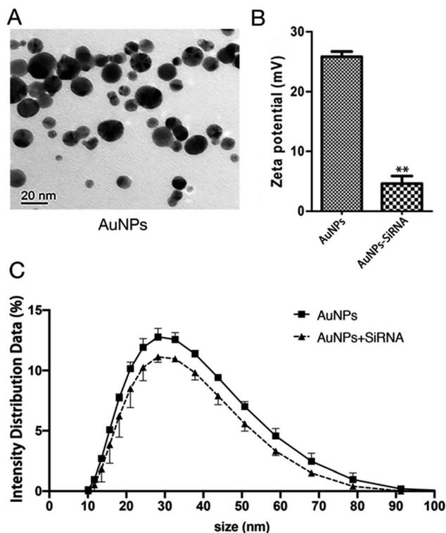
Fig. 3 Synthesis of AuNPs-siRNA<sub>NPR1</sub>. (A) Transmission Electron Microscope (TEM) images of bare AuNPs. Bars = 20 nm. (B) Zeta potential of the AuNPs (left) and siRNA-AuNPs (right). Student's *t*-test (\*,  $p < 0.05$ , \*\*,  $p < 0.01$ , and \*\*\*,  $p < 0.001$ ). (C) The particle size of AuNPs and the change of particle size after AuNPs and siRNA are combined.
