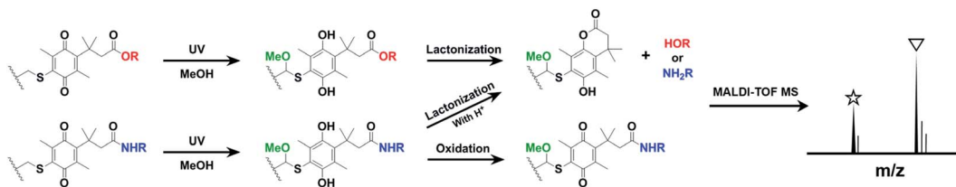
Fig. 1 Schematic of the acid-assisted photochemical release of the trimethyl lock on the surface.
