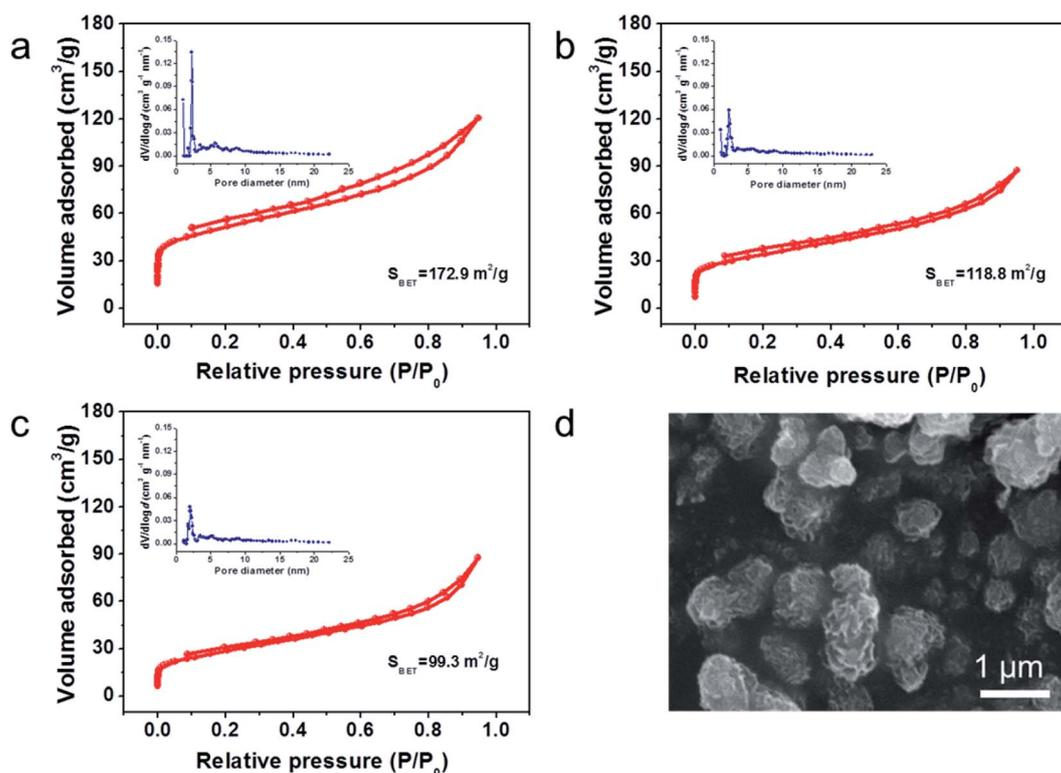
Fig. 3 N<sub>2</sub> adsorption–desorption isotherms results of (a) MHC-1; (b) MHC-2; (c) MHC-3 (inset: pore-size distributions); (d) SEM of MHC/S-2 compound.
