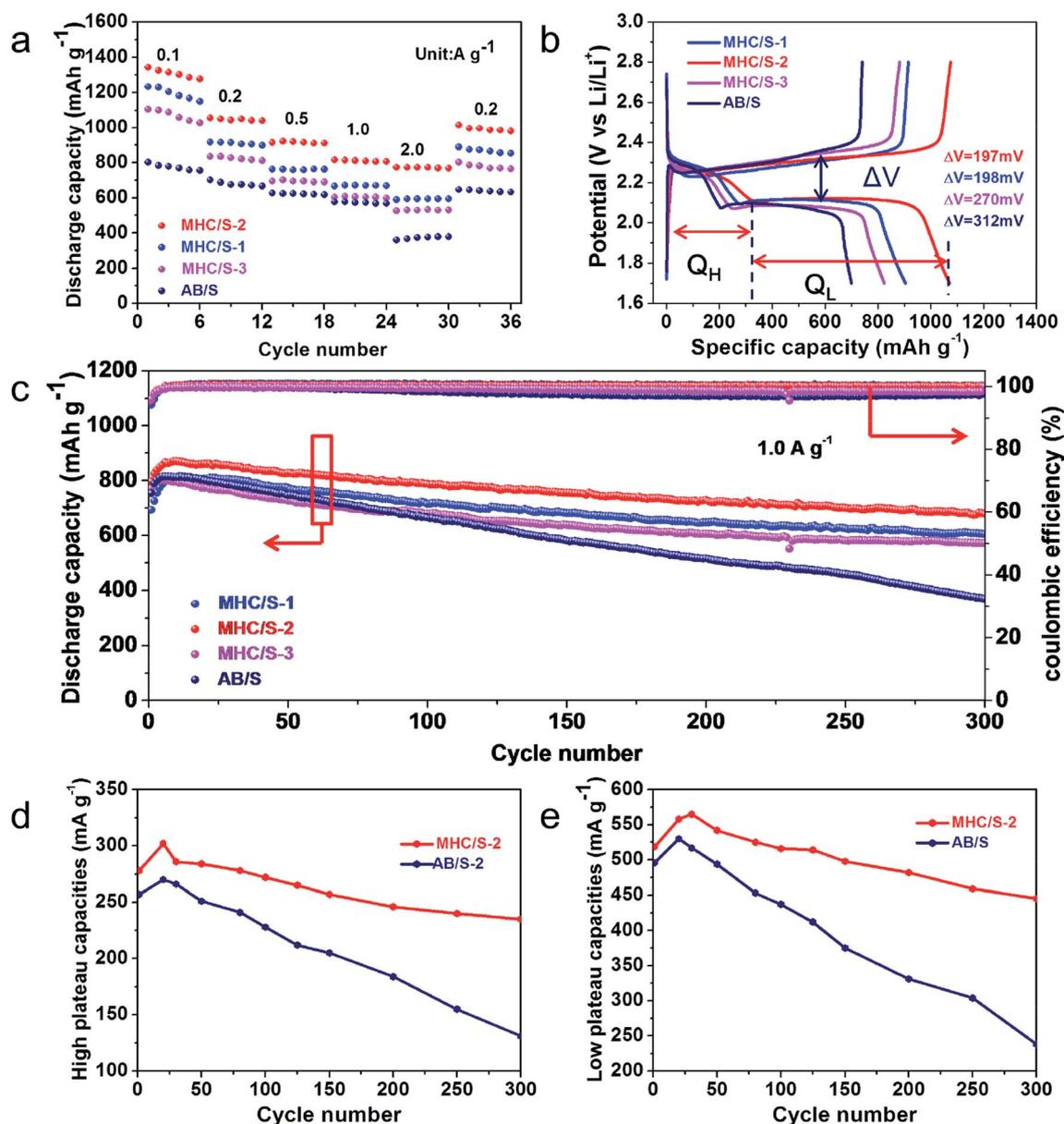
Fig. 5 (a) The rate performance of different cells from 0.1–2 A g<sup>-1</sup>; (b) typical charge–discharge process curve of different cells at 0.2 A g<sup>-1</sup>; (c) cycling performance of different cells at 1.0 A g<sup>-1</sup> for 300 cycles; high plateau (Q<sub>H</sub>) (d) and low plateau (Q<sub>L</sub>) (e) discharge capacities of MHC/S-2 and AB/S at 1.0 A g<sup>-1</sup>.
