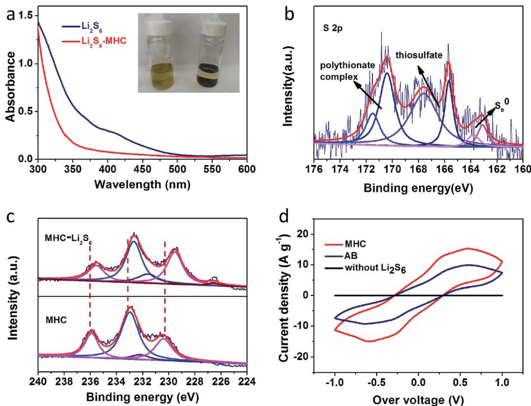
Fig. 8 UV-vis absorption spectra (a) of an  $\text{Li}_2\text{S}_6$  solution before and after immersing MHC-2 (inset: photograph of pure  $\text{Li}_2\text{S}_6$  solution and  $\text{Li}_2\text{S}_6$  solution after immersing MHC-2 for 6 h); high-resolution XPS spectra (b) of S 2p for MHC-2 after adsorption; (c) Mo 3d in pure MHC-2 and MHC-2/ $\text{Li}_2\text{S}_6$ ; (d) cyclic voltammograms of  $\text{Li}_2\text{S}_6$  symmetrical cells employing MHC and AB as working electrodes.
