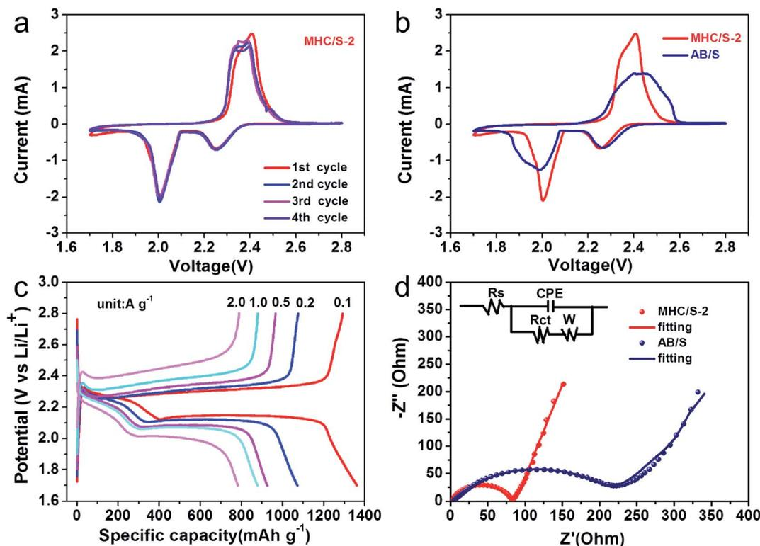
Fig. 6 (a) Cyclic voltammogram curve of MHC/S-2 at a scan rate of  $0.1 \text{ mV s}^{-1}$ ; (b) CV of MHC/S-2 and AB/S at a scan rate of  $0.1 \text{ mV s}^{-1}$ ; (c) the discharge–charge curve in different current density MHC/S-2; (d) EIS of three MHC/S and AB/S before cycle (schematic of equivalent circuit inset).
