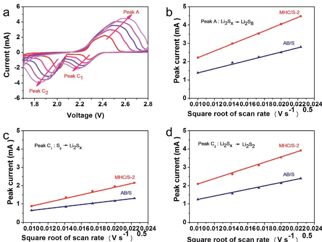
Fig. 7 (a) CV curves of MHC/S electrode from  $0.1$  to  $0.5 \text{ mV s}^{-1}$ ; (b-d) the relationships between the peak current and scan rate in MHC/S-2 and AB/S composites. (b) Peak A:  $\text{S}_8 \rightarrow \text{Li}_2\text{S}_x$ ; (c) peak C<sub>1</sub>:  $\text{Li}_2\text{S}_x \rightarrow \text{Li}_2\text{S}_2/\text{Li}_2\text{S}$ ; (d) peak C<sub>2</sub>:  $\text{Li}_2\text{S}_x \rightarrow \text{S}_8$ .
