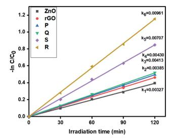
Fig. 6 The kinetics data of ZnO, rGO and ZnO/rGO composites for tetracycline oxidation (120 min of irradiation time, 50 mg  $\rm L^{-1}$  of catalyst, 20 ppm of TC).
