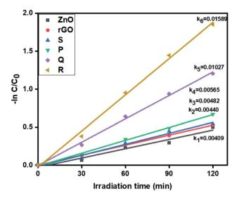
Fig. 7 The kinetic data of ZnO, rGO and ZnO/rGO composites for  $Cr(v_1)$  reduction (120 min of irradiation time, 50 mg  $L^{-1}$  of catalyst, 20 ppm of  $Cr(v_1)$ ).
