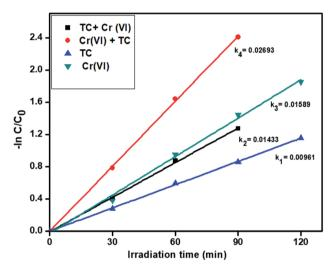
Fig. 8 The kinetics data for the simultaneous removal of TC oxidation and  $Cr(v_i)$  reduction (120 min of irradiation time, 50 mg  $L^{-1}$  of catalyst R, 20 ppm of TC, 20 ppm of  $Cr(v_i)$ , pH = 5 of TC, pH = 4 of  $Cr(v_i)$ ).
