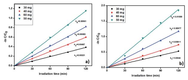
Fig. 10 The kinetic data for effect of catalyst on (a) TC oxidation and (b)  $Cr(v_1)$  reduction (2 h of irradiation time, 20 ppm of TC, 20 ppm of  $Cr(v_1)$ , pH = 5 of TC, pH = 4 of  $Cr(v_1)$ ).
