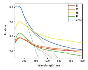
Fig. 3 UV-VIS-DRS spectrum of ZnO and ZnO/rGO composites.
