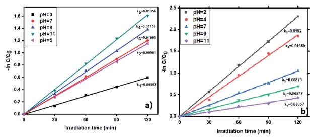
Fig. 11 The kinetic data for effect of pH on (a) TC and (b) Cr(v) with photocatalyst R (2 h of irradiation time, 50 mg  $L^{-1}$  of catalyst, 20 ppm of TC, 20 ppm of Cr(vi)).
