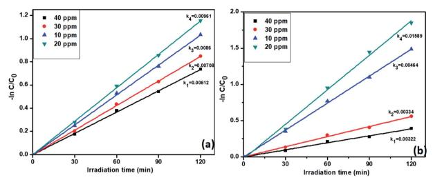
Fig. 9 The kinetic data for the effect of concentration on (a) TC oxidation and (b)  $Cr(v_1)$  reduction with photocatalyst R (2 h of irradiation time, 50 mg L<sup>-1</sup> of catalyst, pH = 5 of TC, pH = 4 of  $Cr(v_1)$ ).
