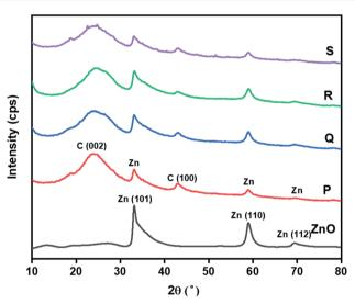
Fig. 1 Powder-XRD patterns of ZnO QD and ZnO/rGO composites
