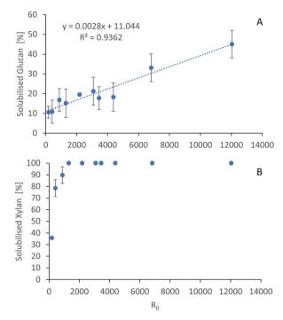
Fig. 4 Polysaccharide dissolution as a function of the severity factors. (A) Glucan. (B) Xylan. Eucalyptus was pretreated at a 1:10~g/g biomass to solvent ratio in  $80\%~[N_{2220}][HSO_4]$  with 20% water.
