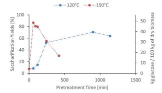
Fig. 3 Glucose yield of pretreated eucalyptus at a 1:10 g/g biomass to solvent ratio in  $80\% \ [N_{2220}][HSO_4]$  with 20 wt% water after enzymatic saccharification.
