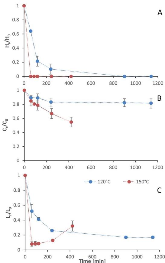
Fig. 2 The mass fraction of (A) hemicellulose [ $H_f/H_0$ ], (B) cellulose [ $C_f/C_0$ ], and (C) lignin [ $L_r/L_0$ ] remaining in the pulp after pretreatment as a function of time at two temperatures (blue line 120 °C, red line 150 °C). Dotted lines were added to guide the reader's eye and are not a kinetic fit. Eucalyptus was pretreated at a 1 : 10 g/g biomass to solvent ratio in 80%  $[N_{2220}][HSO_4]$  with 20 wt% water.
