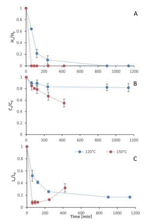
Fig. 2 The mass fraction of (A) hemicellulose  $[H_r/H_0]$ , (B) cellulose  $[C_r/C_0]$ , and (C) lignin  $[L_r/L_0]$  remaining in the pulp after pretreatment as a function of time at two temperatures (blue line 120 °C, red line 150 °C). Dotted lines were added to guide the reader's eye and are not a kinetic fit. Eucalyptus was pretreated at a 1:10 g/g biomass to solvent ratio in 80%  $[N_{2220}][HSO_4]$  with 20 wt% water.
