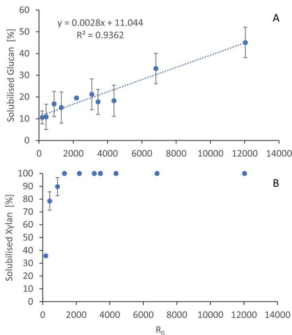
Fig. 4 Polysaccharide dissolution as a function of the severity factors. (A) Glucan. (B) Xylan. Eucalyptus was pretreated at a 1 : 10 g/g biomass to solvent ratio in 80%  $[\text{N}_{2220}][\text{HSO}_4]$  with 20% water.
