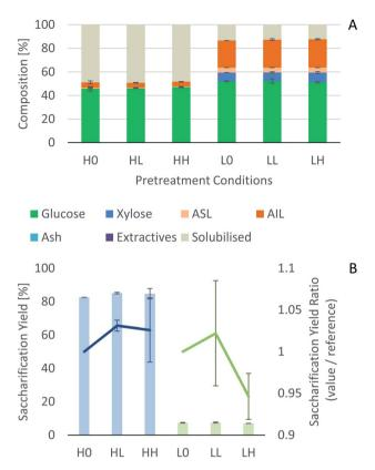
Fig. 6 Effect of CO<sub>2</sub> atmospheres on eucalyptus pretreatment. (A) Pretreated pulp compositions. (B) Saccharification yield of pretreated pulps (bars - left axis) and normalized saccharification yields relative to the control experiments (lines - right axis).
