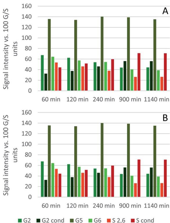
Fig. 9 Abundance of C-H<sub>n</sub> sites on the guaiacyl and syringyl rings of isolated eucalyptus lignin, obtained after pretreatment with [N<sub>2220</sub>][HSO<sub>4</sub>] with 20 wt% water at 120 °C (A) and 150 °C (B).
