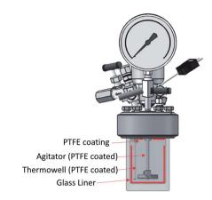
Fig. 10 Schematic representation of the reactor used for the CO<sub>2</sub> atmosphere experiments.
