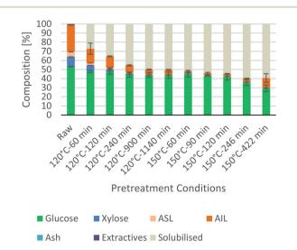
Fig. 1 Eucalyptus pulp composition at different pretreatment conditions using a 1:10 g/g biomass to solvent ratio in 80% [N<sub>2220</sub>][HSO<sub>4</sub>] with 20 wt% water.
