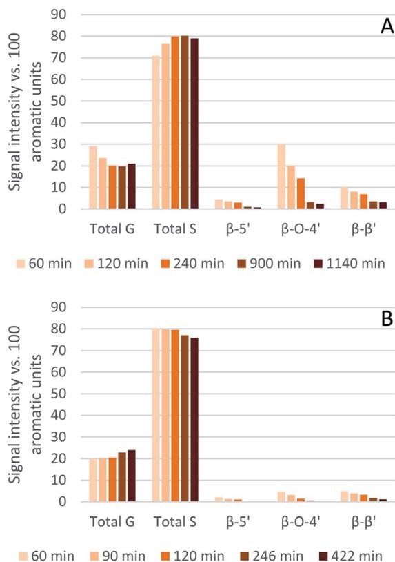
Fig. 8 Abundance of *S* and *G* units and ether linkages of isolated eucalyptus lignin, obtained after pretreatment with [N<sub>2220</sub>][HSO<sub>4</sub>] with 20 wt% water at 120 °C (A) and 150 °C (B).
