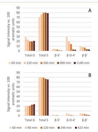
Fig. 8 Abundance of S and G units and ether linkages of isolated eucalyptus lignin, obtained after pretreatment with  $[N_{2220}][HSO_4]$  with 20 wt% water at 120 °C (A) and 150 °C (B).
