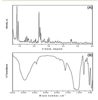
Fig. 1 (A) XRD pattern and (B) IR spectrum of as-synthesized mesoporous  ${\rm HSO_3-ZSM-5}$  zeolite.
