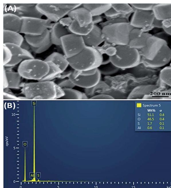
Fig. 2 (A) SEM image and (B) EDS spectrum of as-synthesized HSO<sub>3</sub>-ZSM-5 zeolite.
