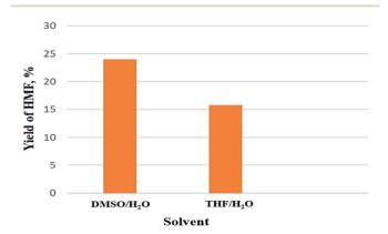
Fig. 3 Effect of solvent on yield of HMF (reaction condition: temperature of 130  $^{\circ}$ C in 2 h with 20% catalyst).
