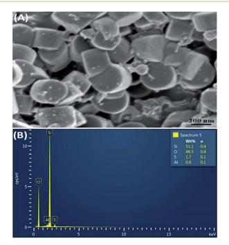
Fig. 2 (A) SEM image and (B) EDS spectrum of as-synthesized  $HSO_3-ZSM-5$  zeolite.
