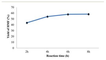
Fig. 6 Effect of reaction time on yield of HMF (reaction condition: temperature of  $140\,^{\circ}\text{C}$  with catalyst dosage of 30%).
