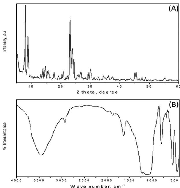
Fig. 1 (A) XRD pattern and (B) IR spectrum of as-synthesized mesoporous HSO<sub>3</sub>-ZSM-5 zeolite.
