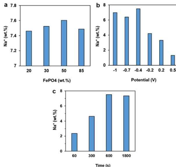
Fig. 3 Effects of (a) FePO<sub>4</sub> loading on the carbon support, (b) electrode potential, and (c) time on the Na<sup>+</sup> capacity of amorphous FePO<sub>4</sub>.
