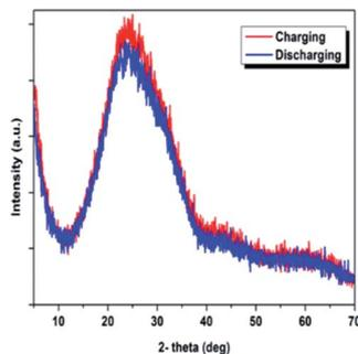
Fig. 7 XRD of the FePO<sub>4</sub> electrode (a) after the charging process at 1.2 V and (b) after the discharging process at 0 V.
