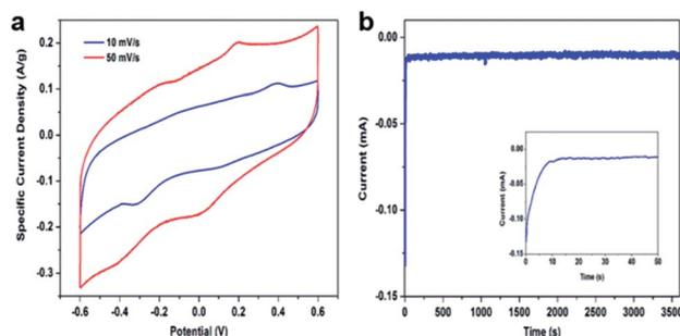
Fig. 2 (a) CV curves of the amorphous FePO<sub>4</sub> in 0.1 M NaCl aqueous solution with a scan rate of 50 mV s<sup>-1</sup> and 10 mV s<sup>-1</sup>, (b) chronoamperometry at -0.4 V vs. Ag/AgCl.
