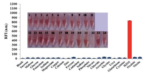
Fig. 5 Fluorescence responses of FLS@MnO $_2$  NS in the presence of different interfering species (300  $\mu$ M of each) at the selected conditions. Inset: photographs (from 1 to 24) corresponding to *X*-axis species of the diagram (from left to right). The concentrations of H $_2$ O $_2$  (2  $\mu$ M), error bars represent the standard deviations of three repetitive experiments.
