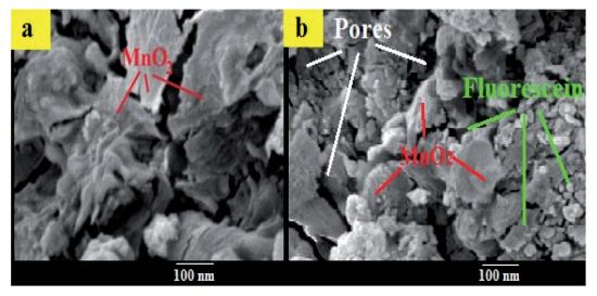
Fig. 3 SEM images of (a) MnO<sub>2</sub> NS (b) FLS@MnO<sub>2</sub> NS.
