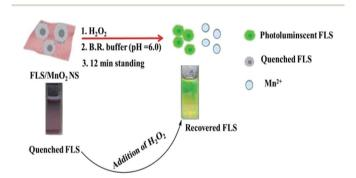
Scheme 2 Principle for H<sub>2</sub>O<sub>2</sub> detection using FLS@MnO<sub>2</sub> NS.
