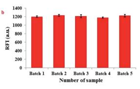
Fig. 6 Homogeneity of FLS@MnO<sub>2</sub> NS and reproducibility of the synthesis procedure assessed by (a) spectrophotometric determination at 495 nm of five independent batches and (b) fluorescence detection of 3  $\mu$ M H<sub>2</sub>O<sub>2</sub> at five independent batches of FLS@MnO<sub>2</sub> NS.
