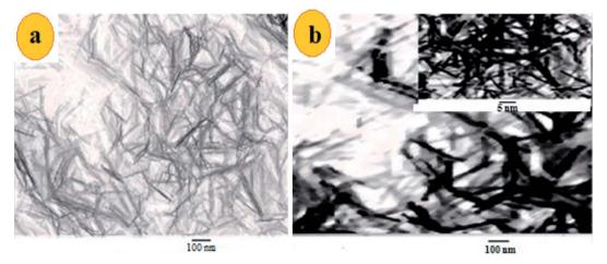
Fig. 2 TEM images of (a) ultrathin MnO<sub>2</sub> NS and (b) FLS@MnO<sub>2</sub> nanocomposite at 100 nm and inset of (b) is a higher magnification.
