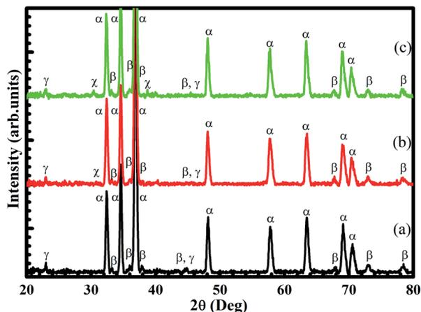
Fig. 1 X-ray diffraction (XRD) results of (a) Mg-5Al-4Sn-based, (b) Mg-5Al-4Sn-0.5Sr and (c) Mg-5Al-4Sn-1.0Sr alloys ( $\alpha$ -Mg,  $\beta$ -Mg<sub>17</sub>Al<sub>12</sub>,  $\gamma$ -Mg<sub>2</sub>Sn and  $\chi$ -MgAlSr).
