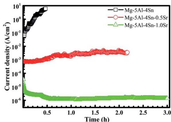
Fig. 6 Changes in current density as a function of time under a constant applied anodic potential of 800 mV<sub>SCE</sub>.
