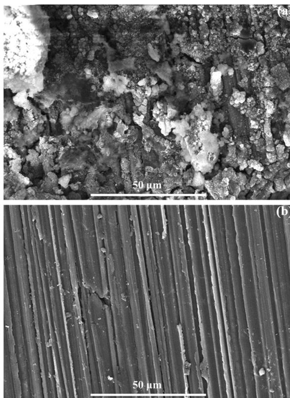
Fig. 7 SEM images of (a) Mg-5Al-4Sn and (b) Mg-5Al-4Sn-1.0Sr alloys after applying a constant anodic potential of 800 mV<sub>SCE</sub>.
