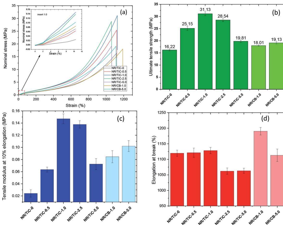
Fig. 1 (a) Nominal stress vs. strain (%) (b) maximum tensile strength of the composites (c) tensile modulus at 10% elongation and (d) elongation at break of the prepared composites.
