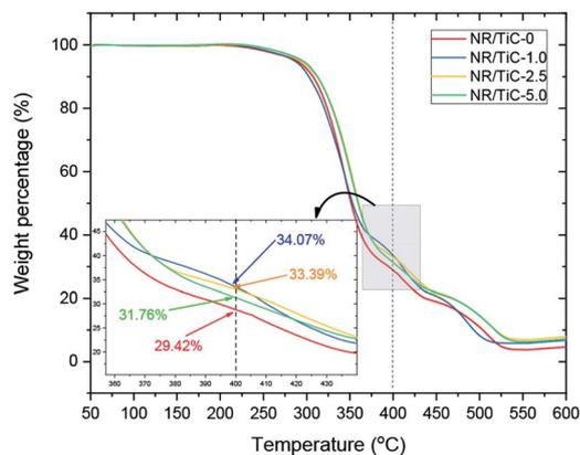
Fig. 6 Thermogravimetric analysis of the TiC rubber nanocomposites.
