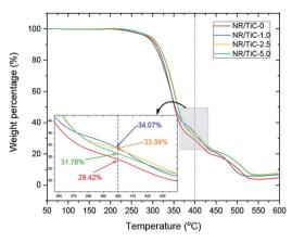
Fig. 6 Thermogravimetric analysis of the TiC rubber nanocomposites
