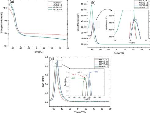
Fig. 3 Dynamic mechanical analysis: (a) storage modulus (b) loss modulus (c) and tan delta of the prepared rubber composites.
