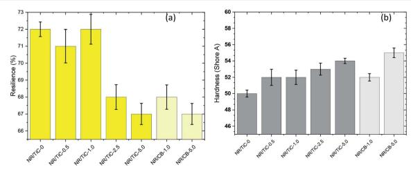
Fig. 2 (a) Resilience and (b) hardness of the prepared TiC/NR rubber composites
