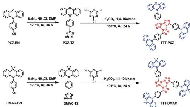
Scheme 1 The synthetic routes for TTT-PXZ and TTT-DMAC.
