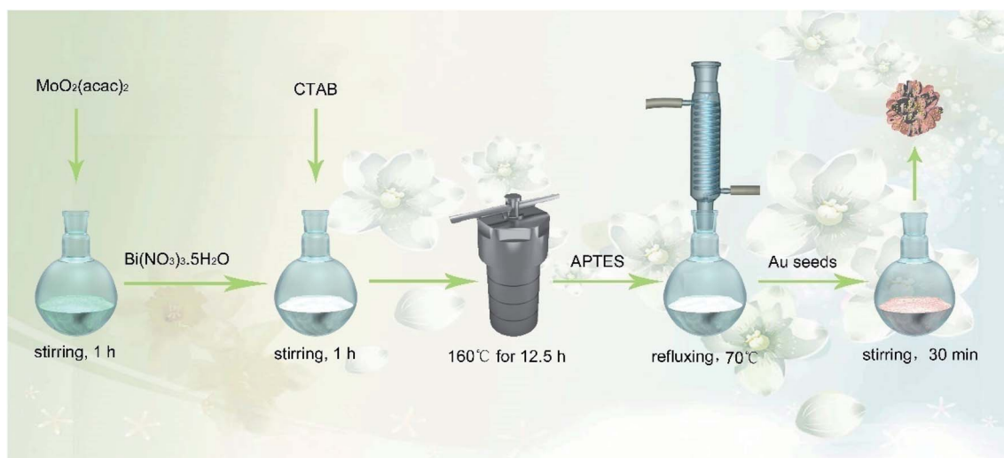
Scheme 2 The schematic for the synthesis of Au@Bi 2 MoO 6 NTs.
