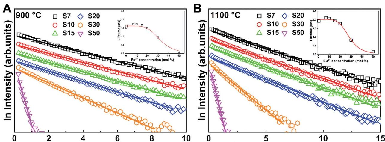
Fig. 7 PL decay curves for curves for the  $\text{Eu}^{3+} {}^5\text{D}_0$  excited state under excitation at CTB of  $\text{Eu}^{3+}$  doped  $\text{Y}_3\text{TaO}_7$  samples annealed at (A) 900 or (B) 1100 °C with fixed emission at 607.0 nm. Inset: lifetime values ( $\tau_{\text{obs}}$ ) as a function of  $\text{Eu}^{3+}$  concentration (from 0.1 [30] up to 50 mol%) under excitation at CTB. The lines are visual guides.
