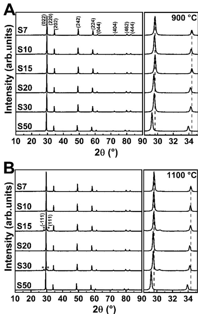
Fig. 1 X-ray diffractograms of  $Eu^{3+}$ -doped  $Y_3TaO_7$  samples annealed at (A) 900 or (B) 1100 °C for 2 h. The  $M'-YTaO_4$  phase planes are marked (\*). At the right side, a magnification in the region of 28–35° and  $2\theta$  shift is observed.
