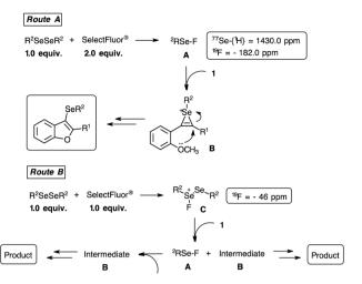
**Scheme 7** Plausible mechanism routes for the synthesis of 3-organ-ylselanyl-benzo[*b*] furans **3**.
