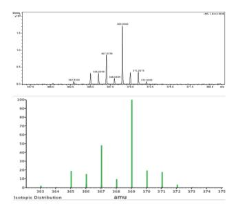
Fig. 2 HRMS and isotopic distribution of product 4a (up: experimental analysis; and down: calculated MW + Na<sup>+</sup> = 369.0369).
