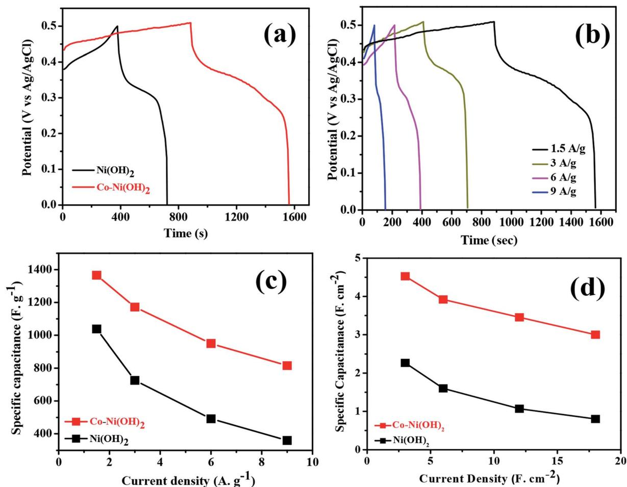
Fig. 7 (a) GCD curves of Ni(OH)<sub>2</sub> and Co–Ni(OH)<sub>2</sub> composites measured at 1.5 A g<sup>−1</sup>, (b) GCD cycling profile of Co–Ni(OH)<sub>2</sub> evaluated at different current densities, (c) gravimetric (d) volumetric specific capacitance of Co–Ni(OH)<sub>2</sub>, Ni(OH)<sub>2</sub> electrodes at various current densities.
