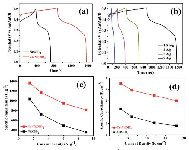
Fig. 7 (a) GCD curves of Ni(OH)<sub>2</sub> and Co-Ni(OH)<sub>2</sub> composites measured at 1.5 A  $g^{-1}$ , (b) GCD cycling profile of Co-Ni(OH)<sub>2</sub> evaluated at different current densities, (c) gravimetric (d) volumetric specific capacitance of Co-Ni(OH)<sub>2</sub>, Ni(OH)<sub>2</sub> electrodes at various current densities.
