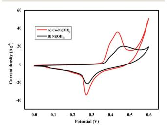
Fig. 6 Cyclic voltammetry behaviors of (A)  $Co-Ni(OH)_2$  (B)  $Ni(OH)_2$  electrodes at the same scan rate of 10 mV s<sup>-1</sup>.
