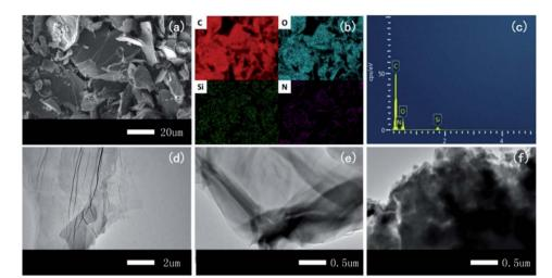
Fig. 4 (a) SEM image of FR-fGO with (b) elemental mapping of C, O, Si, and N and (c) EDX results of FR-fGO. TEM patterns of (d) GO, (e) I-GO, and (f) FR-fGO
