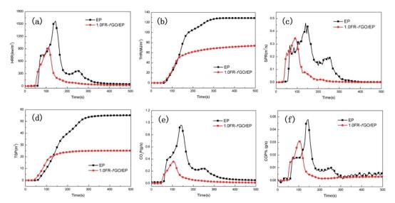
Fig. 5 HRR (a), THR (b), SPR (c), and TSP (d) vs. time curves of EP and its composites. CO (e) and CO<sub>2</sub> (f) yields vs. EP and its composites.
