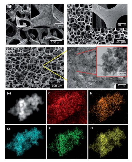
Fig. 4 FESEM images of (a) 3DG on Ni foam, (b) Ni etched 3DG foam, (c) HAp anchored N3DG ceramic framework, (d) TEM image of HAp-N3DG, and (e) elemental mapping of HAp-N3DG.
