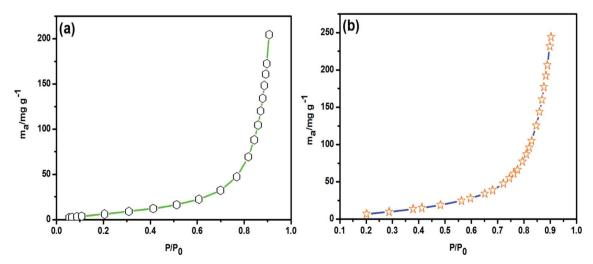
Fig. 8 Adsorption graphs of HAp-N3DG nanostructured CF for (a) benzene and (b) toluene adsorption.
