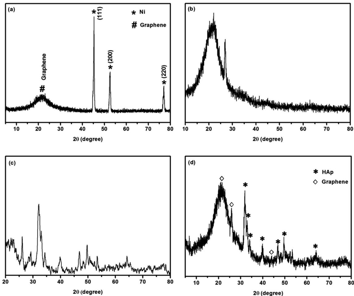
Fig. 2 XRD patterns of (a) 3D graphene on Ni foam, (b) Ni-etched 3D graphene foam, (c) pure hydroxyapatite, (d) hydroxyapatite on N-doped 3D graphene nanostructured ceramic framework.
