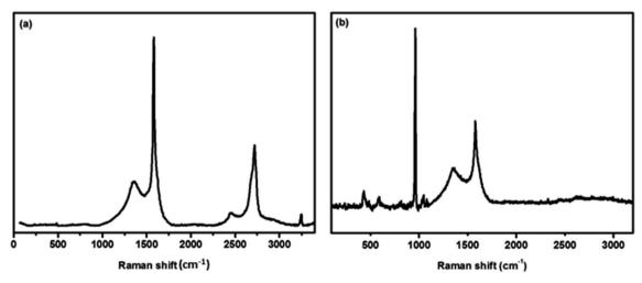
Fig. 3 Raman spectra of (a) commercial 3D graphene on Ni foam and (b) HAp anchored N3DG nanostructured CF.
