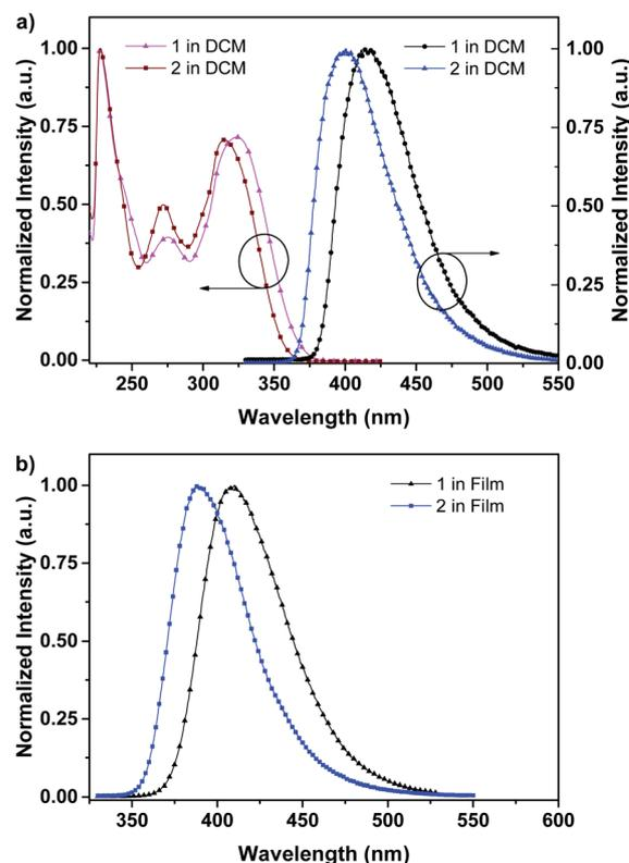
Fig. 1 (a) UV-visible absorption (left), photoluminescence (right) spectra of **1** and **2** in CH<sub>2</sub>Cl<sub>2</sub> at 298 K; (b) photoluminescence spectra of **1** and **2** in film at 298 K.
