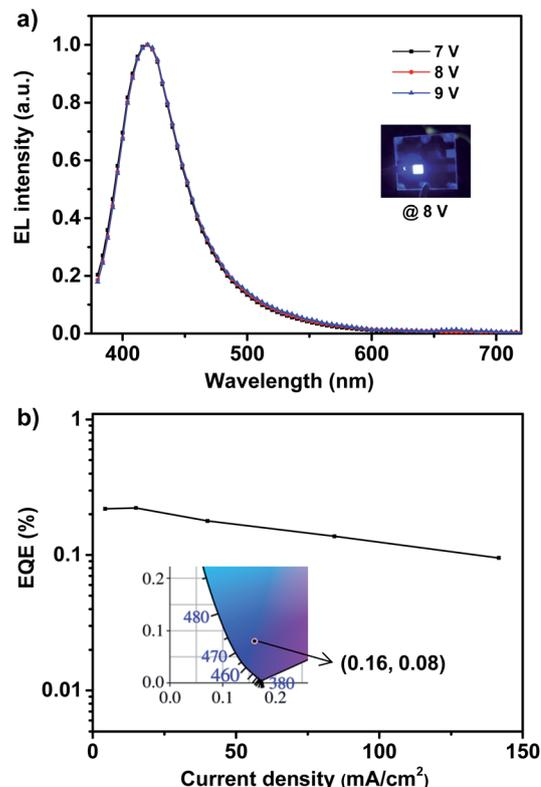
Fig. 3 The EL spectra (a) and EQE- $J$  curve (b) of violet/deep-blue OLED based on **1**. Inset: EL photograph (up) and 1931 CIE coordinate (down) of device at 8 V.
