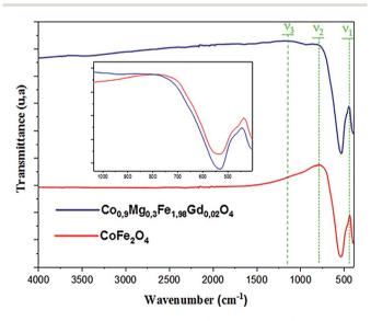
Fig. 4 FTIR spectra of samples  $Co_{0.7}Mg_{0.3}Fe_{1.98}Gd_{0.02}O_4$  and  $CoFe_2O_4$ .
