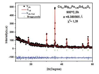
Fig. 3 Typical Rietveld-refined XRD pattern for the  $\rm Co_{0.7}Mg_{0.3}Fe_{1.98}\text{-}Gd_{0.02}O_4$  sample.
