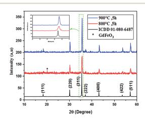
Fig. 1  $\,$  XRD patterns of Co $_{0.7} Mg_{0.3} Fe_{1.98} Gd_{0.02} O_4$  calcined at 800 and 900  $^{\circ} C.$
