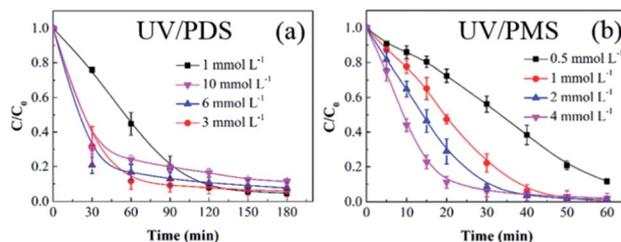
Fig. 2 Effects of the oxidant dose on HA removal in UV/PDS (a) and UV/PMS (b). Conditions: [HA]<sub>0</sub> = 15 mg L<sup>-1</sup>, [PDS]<sub>0</sub> = 1–10 mmol L<sup>-1</sup>, [PMS]<sub>0</sub> = 0.5–4 mmol L<sup>-1</sup>, pH<sub>0</sub> = 6 and 3 for UV/PDS and UV/PMS, respectively.
