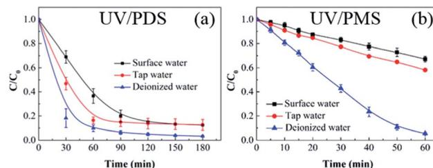
Fig. 7 HA removal from different water sources by UV/PDS (a) and UV/PMS (b). Conditions:  $[HA]_0 = 15 \text{ mg L}^{-1}$ ,  $[PDS]_0 = 3 \text{ mmol L}^{-1}$ ,  $[PMS]_0 = 1 \text{ mmol L}^{-1}$ ,  $\text{pH}_0 = 3.0, 7.4$ , and  $7.8$  for deionized water, surface water, and tap water, respectively.
