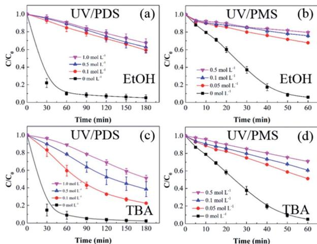
Fig. 4 Effects of radical scavengers on HA removal in UV/PDS (a and c) and UV/PMS (b and d). Conditions:  $[HA]_0 = 15 \text{ mg L}^{-1}$ ,  $[PDS]_0 = 3 \text{ mmol L}^{-1}$ ,  $[PMS]_0 = 1 \text{ mmol L}^{-1}$ ,  $\text{pH}_0 = 6$  and  $3$  for UV/PDS and UV/PMS, respectively.
