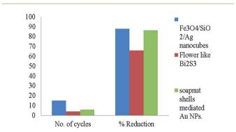
Fig. 6 Comparison based on the recyclability of various catalysts used for 4-NA reduction.  $^{31,44,50}$
