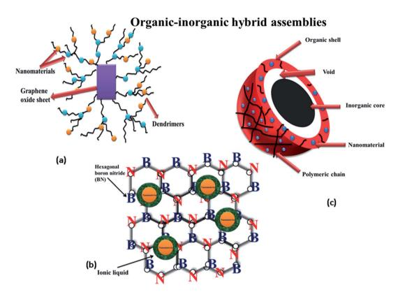
Fig. 4 Organic–inorganic composite nanocatalytic assemblies: (a) dendrimer and graphene supported nanomaterial, (b) hexagonal boron nitride containing nanomaterials and ionic liquid, (c) core–shell microgel.
