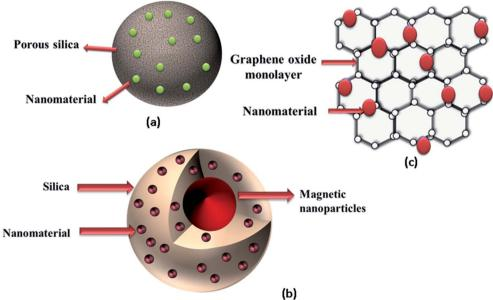
Fig. 2 Inorganic supporting nanocatalytic assemblies: (a) metal nanoparticles impregnated on porous silica, (b) nanomaterial-decorated silicacoated magnetic nanoparticles, (c) graphene oxide sheet containing nanomaterial.
