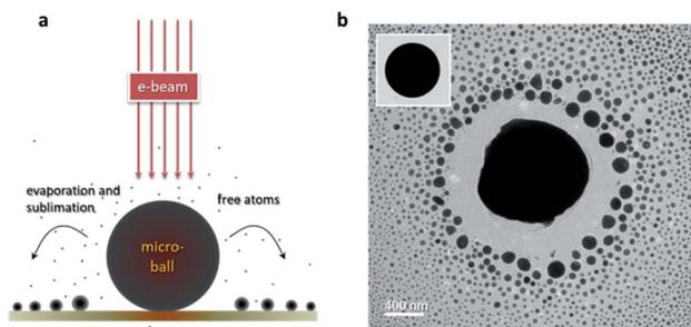
Fig. 1 (a) Schematic illustration of the *in situ* EAD method. (b) Morphology of the alloy nanoparticles formed by the *in situ* EAD method. The inset shows the initial micro-ball before e-beam irradiation.
