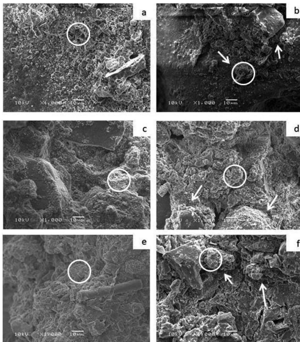
**Fig. 6** SEM micrographs of tested soil samples; (a) sand sample amended with alginate beads (control), (b) calcareous soil sample amended with alginate beads (control), (c) clay soil sample amended with alginate beads (control), (d) sand sample amended with bacterial-immobilized beads, (e) calcareous soil sample amended with bacterial-immobilized beads, and (f) clay soil sample amended with bacterial-immobilized beads.
