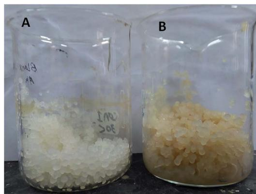
Fig. 1 Calcium alginate beads (A) without bacteria, and (B) with bacteria.
