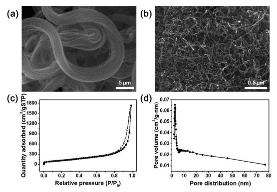
Fig. 2 (a and b) SEM images of commercial CNTs. (c) Nitrogen adsorption-desorption isotherms and (d) pore distribution of commercial CNTs.
