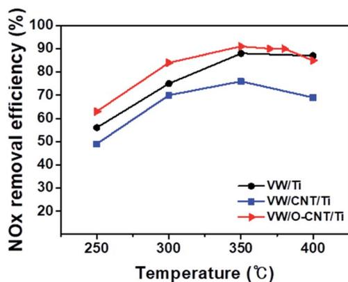
Fig. 6 NO<sub>x</sub> removal efficiencies\* of synthesized VW/Ti, VW/CNT/Ti, and VW/O-CNT/Ti catalysts as a function of temperature from 250 to 400 °C. \*Catalytic reaction conditions: [NO<sub>x</sub>] = 500 ppm, [NH<sub>3</sub>] = 500 ppm, [O<sub>2</sub>] = 5%, balance gas N<sub>2</sub>, total flow 500 sccm, and GHSV = 300 000 ml gcat<sup>-1</sup> h<sup>-1</sup>.
