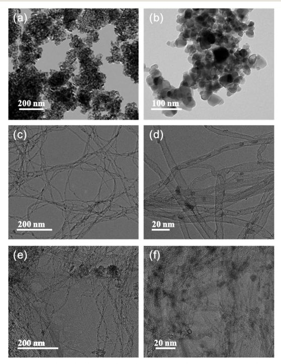
Fig. 4 TEM images of synthesized (a and b) VW/Ti catalyst, (c and d) V-W impregnated O-CNT nanocomposite, and (e and f) VW/O-CNT/Ti catalyst.
