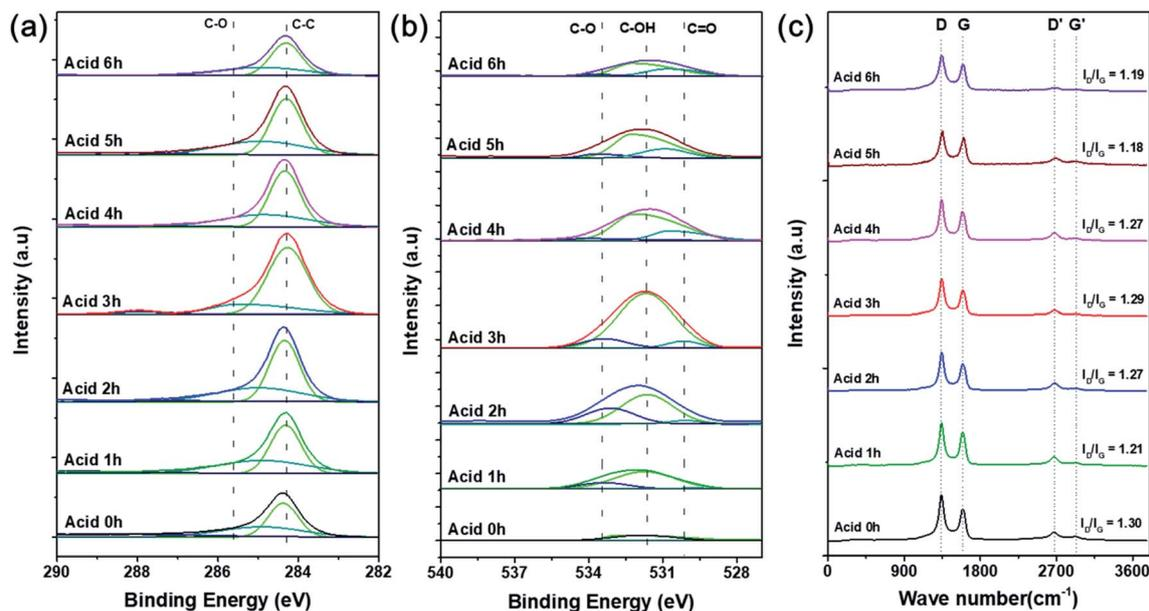
Fig. 3 Deconvoluted (a) C 1s and (b) O 1s XPS curves and (c) Raman spectra of O-CNTs prepared with various acid treatment times.
