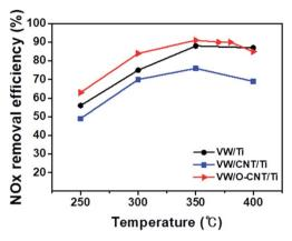
Fig. 6 NO $_{x}$  removal efficiencies\* of synthesized VW/Ti, VW/CNT/Ti, and VW/O-CNT/Ti catalysts as a function of temperature from 250 to 400 °C. \*Catalytic reaction conditions: [NO $_{x}$ ] = 500 ppm, [NH $_{3}$ ] = 500 ppm, [O $_{2}$ ] = 5%, balance gas N $_{2}$ , total flow 500 sccm, and GHSV = 300 000 ml gcat $^{-1}$  h $^{-1}$ .
