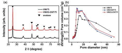
(a) XRD patterns and (b) pore size distributions of the synthesized SCR catalysts.
