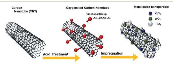
$\textbf{Fig. 1} \quad \textbf{Schematic diagram of the synthesis of O-CNTs and V-W-Ti-doped CNT SCR catalysts } \\$
