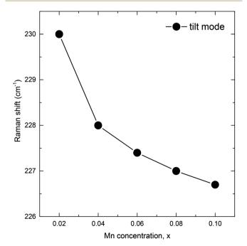
Fig. 6 Position of the  $A_1$ -2(TO) tilt mode as a function of Mn concentration.
