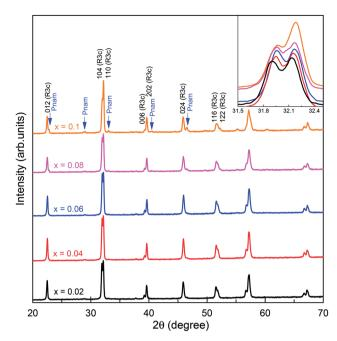
Fig. 1 XRD patterns of  $Bi_{0.88}Sm_{0.12}Fe_{1-x}Mn_xO_3$  (BSFMO) samples. The inset shows the diffraction peaks at around 32°.
