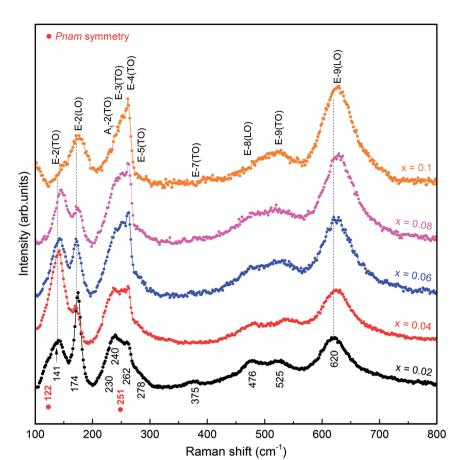
Fig. 4 Raman scattering (RS) spectra of BSFMO samples.
