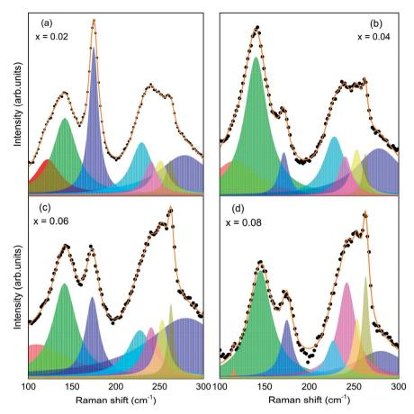
Fig. 5 Typical deconvoluted Raman spectra for (a) x = 0.02, (b) x = 0.04, (c) x = 0.06, and (d) x = 0.08 in the region of 100-300 cm<sup>-1</sup>.
