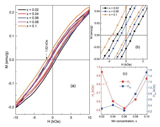
Fig. 7 (a) M(H) loops of BSFMO samples measured immediately after synthesis. (b) The enlarged view around the origin of x = 0.02, 0.06, and 0.10 samples. (c) The  $H_c$  and  $H_{eb}$  as a function of Mn concentration.
