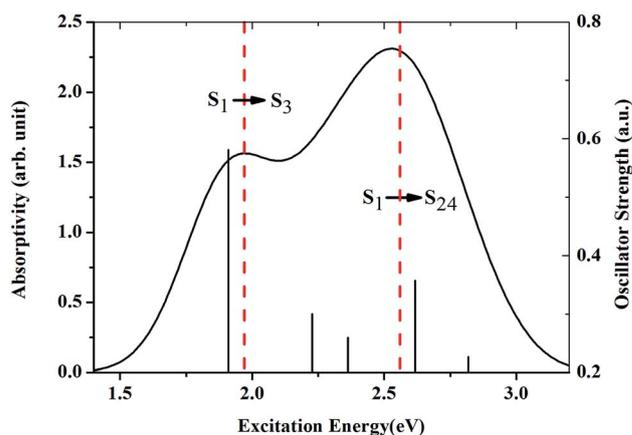
Fig. 2 Simulated absorption spectrum for ZnPc in the first singlet excited state ( $S_1$ ), which is in good agreement with the experimental results. The red dashed lines are the two peaks of the spectrum observed in the experiment.
