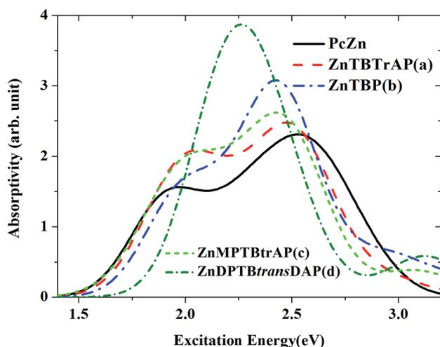
Fig. 7 Comparison of the absorption spectra of ZnPc and modified ZnPc in the first singlet excited state ( $S_1$ ). The spectra are described using the calculated oscillator strengths and excitation energies broadened with the Gaussian function (FWHM = 0.4 eV).
