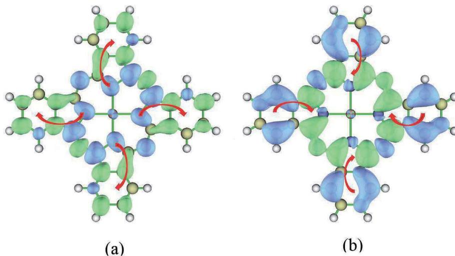
Fig. 5 Electron density difference of ZnPc for  $S_1 \rightarrow S_3$  and  $S_1 \rightarrow S_{24}$  transitions. Blue and green regions show a decrease and increase of electron density, respectively. The wavefunction analysis program Multiwfn<sup>30</sup> was used for this analysis. The isosurface values are fixed to  $0.0005 \text{ \AA}^{-3}$ . (a)  $S_1 \rightarrow S_3$ ,  $\Delta\rho = \rho_3(r) - \rho_1(r)$ ; (b)  $S_1 \rightarrow S_{24}$ ,  $\Delta\rho = \rho_{24}(r) - \rho_1(r)$ .
