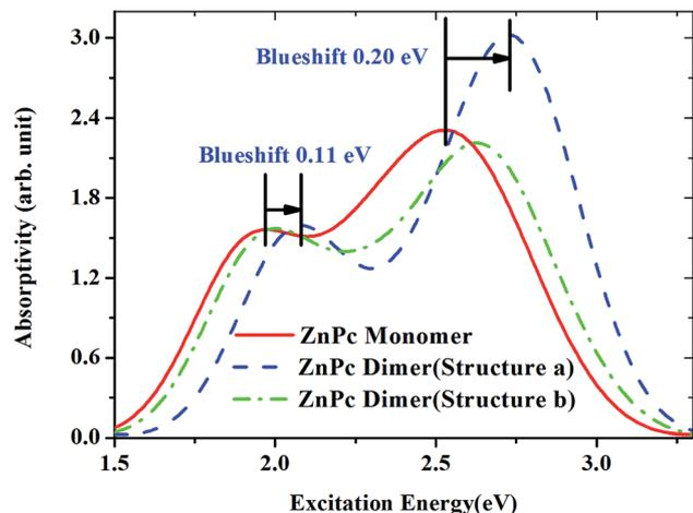
Fig. 9 Comparison of the absorption spectra of ZnPc and ZnPc dimers in the first singlet excited state ( $S_1$ ). The spectra are described using the calculated oscillator strengths and excitation energies broadened with the Gaussian function (FWHM = 0.4 eV).
