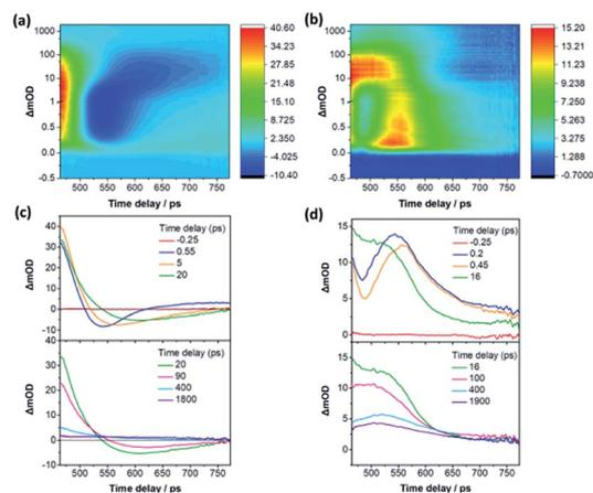
Fig. 4 TA spectra of C1 (a) and C2 (b) diluted in DMSO at excitation wavelength of 400 nm. (c and d) Plots of the TA spectra at various time delays of C1 and C2, respectively.
