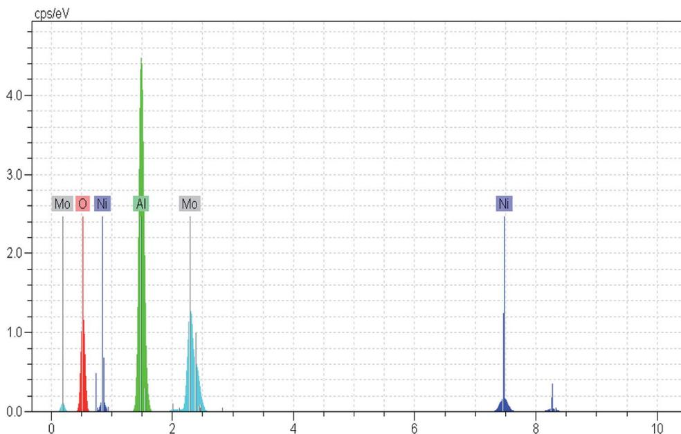
Fig. 2 EDX analysis of NiMo/Al<sub>2</sub>O<sub>3</sub> prepared with combustion synthesis method with fuel/nitrate = 4.
