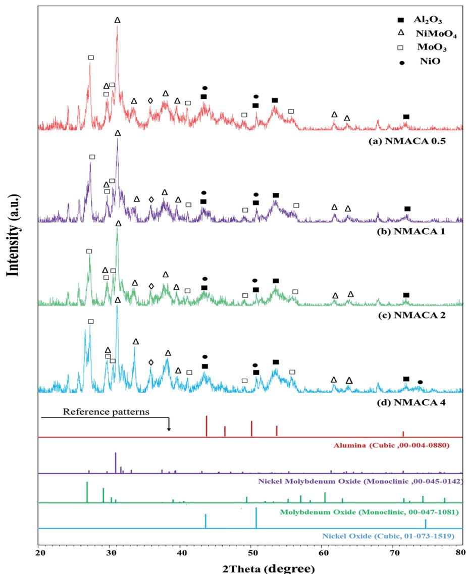
Fig. 1 XRD patterns of NiMo/Al<sub>2</sub>O<sub>3</sub> catalysts with various fuel content (a) NMACA0.5 (b) NMACA1 (c) NMACA2 (d) NMACA4.
