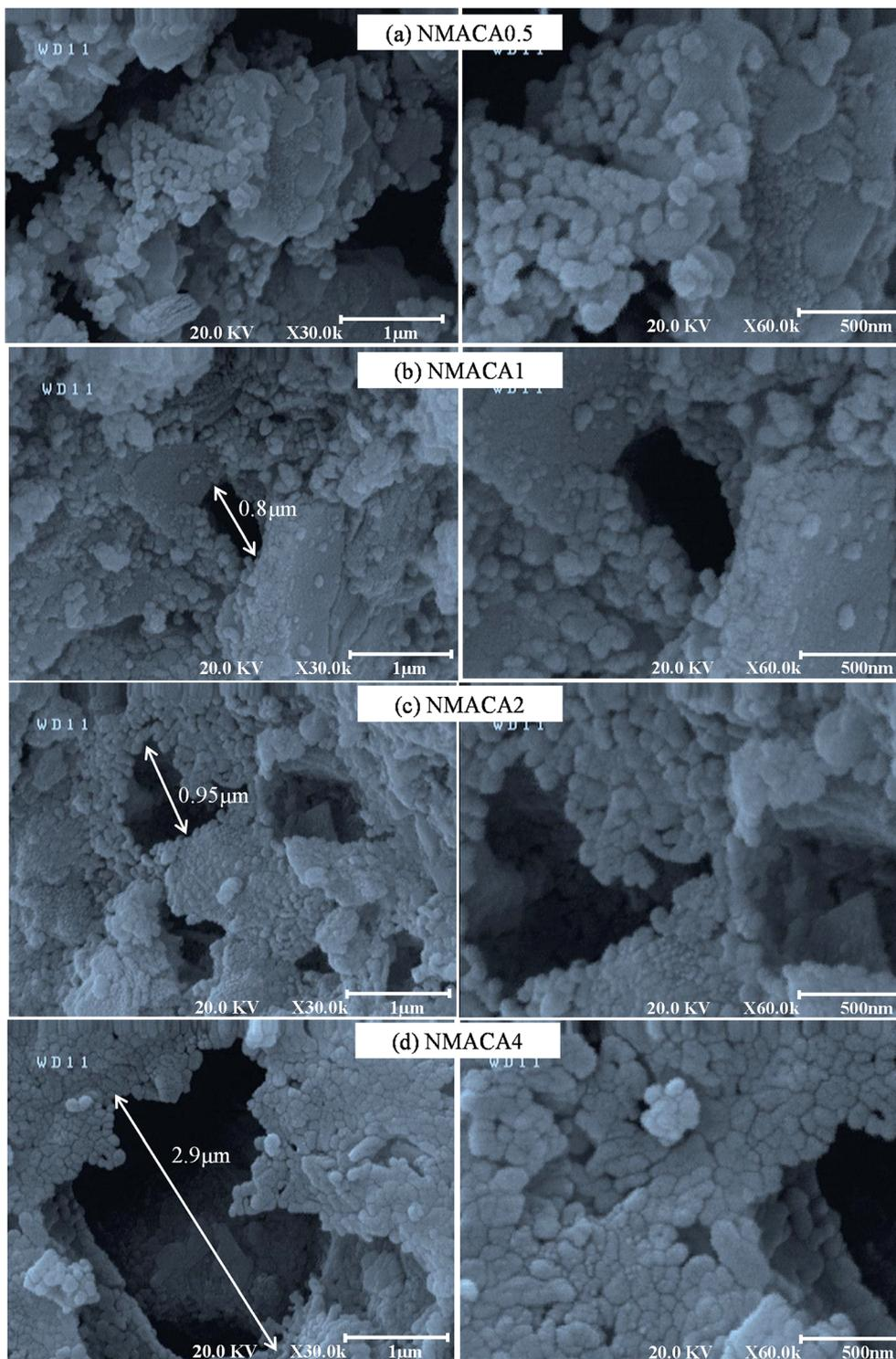
Fig. 4 FESEM images of NiMo/Al<sub>2</sub>O<sub>3</sub> catalysts synthesized with various fuel content (a) NMACA0.5, (b) NMACA1, (c) NMACA2, (d) NMACA4.
