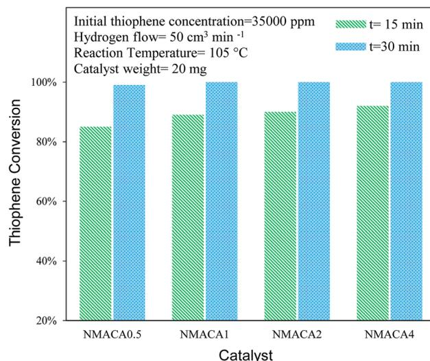
Fig. 9 Catalytic activity of NiMo/Al<sub>2</sub>O<sub>3</sub> with various fuel content toward hydrodesulfurization of thiophene at 105 °C.
