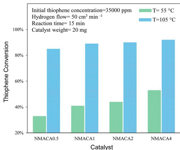
Fig. 8 Catalytic activity of NiMo/Al<sub>2</sub>O<sub>3</sub> with various fuel content toward hydrodesulfurization of thiophene at 15 min.
