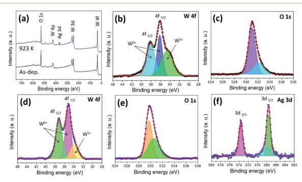
Fig. 7 X-ray photoelectron spectra of the  $WO_3/Ag-WO_3$  films and peak fitting: wide-scan spectra of as-deposited and annealed films (a), high-resolution scan of W and O for as-deposited films (b and c), high-resolution scan of W, O, and Ag for annealed films at 923 K (d, e, and f).
