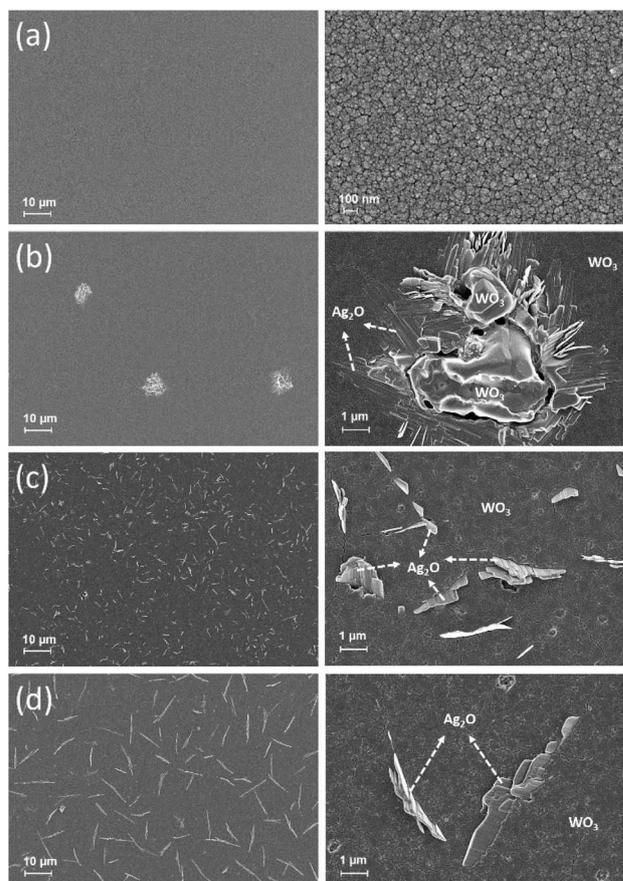
Fig. 3 High ( $10k\times$ ) and low-magnification ( $1k\times$ ) FESEM images of as-deposited and annealed  $\text{WO}_3/\text{Ag-WO}_3$  thin films surface morphology: (a) as-deposited, (b) 823 K, (c) 873 K, and (d) 923 K.
