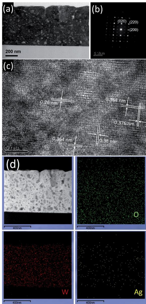
Fig. 5 TEM images of  $\text{WO}_3/\text{Ag}-\text{WO}_3$  films annealed at 923 K: (a) cross-sectional microstructure, (b) SAED pattern of  $\text{WO}_3$ , (c) HR-TEM image with clear crystalline planes of monoclinic- $\text{WO}_3$  phase, and (d) DF STEM image and corresponding EDX elemental distribution of W, O, and Ag.
