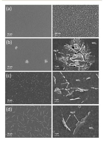
Fig. 3 High ( $10k\times$ ) and low-magnification ( $1k\times$ ) FESEM images of asdeposited and annealed WO<sub>3</sub>/Ag–WO<sub>3</sub> thin films surface morphology: (a) as-deposited, (b) 823 K, (c) 873 K, and (d) 923 K.
