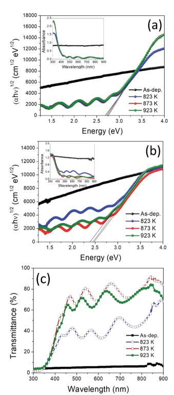
Fig. 6  $(\alpha h \nu)^{1/2}$  vs.  $h \nu$  plots and absorbance spectra of the WO<sub>3</sub> films (a), and WO<sub>3</sub>/Ag–WO<sub>3</sub> films (b); optical transmittance spectra of the asdeposited and annealed WO<sub>3</sub>/Ag–WO<sub>3</sub> films (c).
