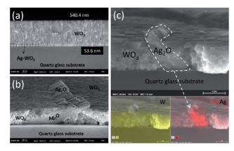
Fig. 4 FESEM images of  $WO_3/Ag-WO_3$  thin films: (a) cross-section of the as-deposited films, (b) cross-section of the annealed films at 923 K, (c) cross-section of backscattering image and EDS elemental mapping of W and Ag corresponding to the annealed films at 923 K.
