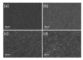
Fig. 2 FESEM images (magnification:  $50k\times$ ) of as-deposited and annealed WO $_3$  thin films surface morphology: (a) as-deposited, (b) 823 K, (c) 873 K, and (d) 923 K.
