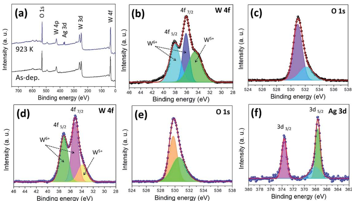
Fig. 7 X-ray photoelectron spectra of the  $\text{WO}_3/\text{Ag}-\text{WO}_3$  films and peak fitting: wide-scan spectra of as-deposited and annealed films (a), high-resolution scan of W and O for as-deposited films (b and c), high-resolution scan of W, O, and Ag for annealed films at 923 K (d, e, and f).
