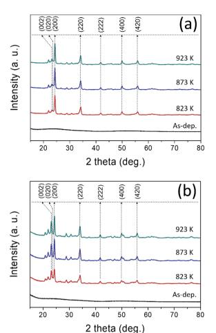
Fig. 1  $\,$  X-ray diffraction patterns of the (a)  $\,$  WO $_3$ /quartz glass, (b)  $\,$  WO $_3$ /Aq-WO $_3$ /quartz glass.
