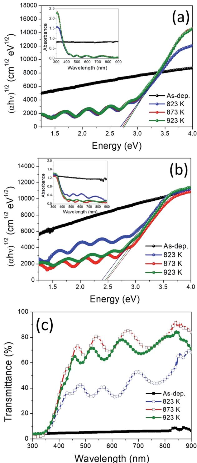
Fig. 6  $(\alpha h\nu)^{1/2}$  vs.  $h\nu$  plots and absorbance spectra of the  $\text{WO}_3$  films (a), and  $\text{WO}_3/\text{Ag}-\text{WO}_3$  films (b); optical transmittance spectra of the as-deposited and annealed  $\text{WO}_3/\text{Ag}-\text{WO}_3$  films (c).
