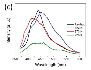
Fig. 8 (a) Photocatalytic performance of the  $WO_3$  and  $WO_3/Ag-WO_3$  films, photodegradation of methylene blue under the irradiation of visible light; the reaction rate constants were calculated based on the pseudo-first-order reaction kinetics. (b) Schematic illustration of the photocatalytic mechanism of  $Ag_2O/WO_3$  p-n heterojunction photocatalyst, and (c) photoluminescence emission spectra of the  $WO_3/Ag-WO_3$  films.
