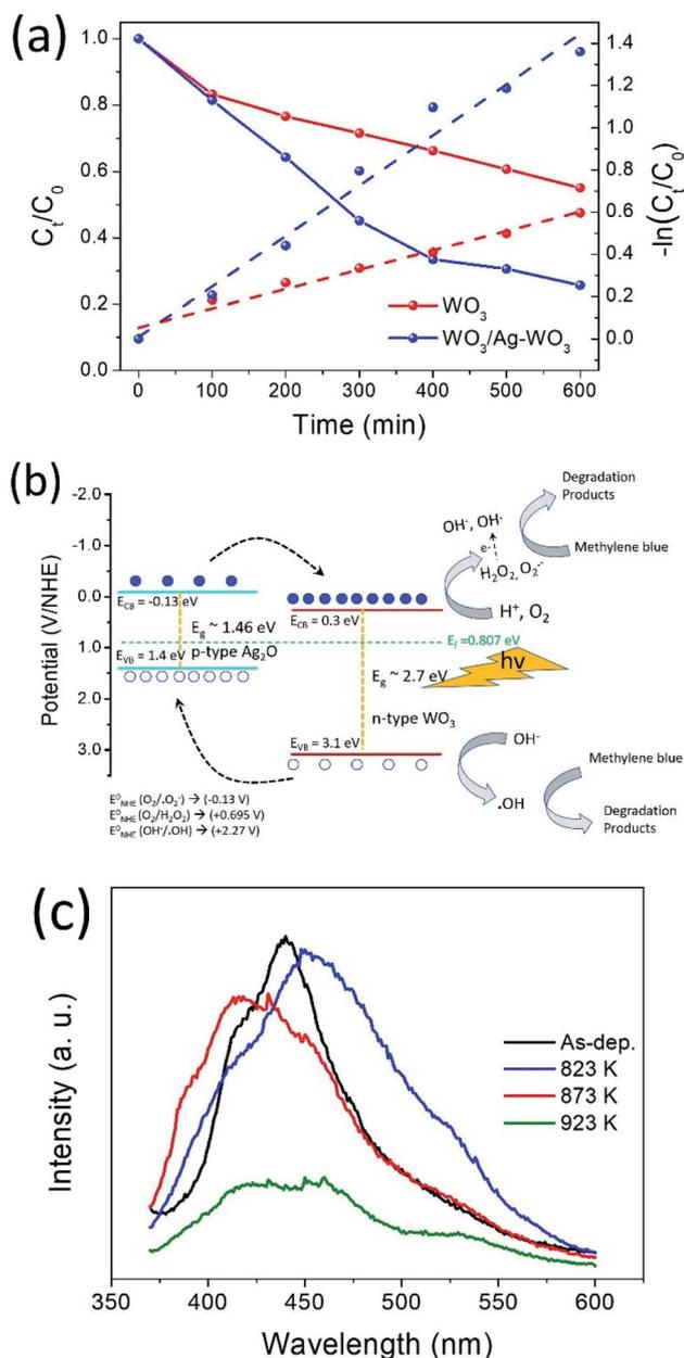
**Fig. 8** (a) Photocatalytic performance of the  $\text{WO}_3$  and  $\text{WO}_3/\text{Ag-WO}_3$  films, photodegradation of methylene blue under the irradiation of visible light; the reaction rate constants were calculated based on the pseudo-first-order reaction kinetics. (b) Schematic illustration of the photocatalytic mechanism of  $\text{Ag}_2\text{O}/\text{WO}_3$  p-n heterojunction photocatalyst, and (c) photoluminescence emission spectra of the  $\text{WO}_3/\text{Ag-WO}_3$  films.
