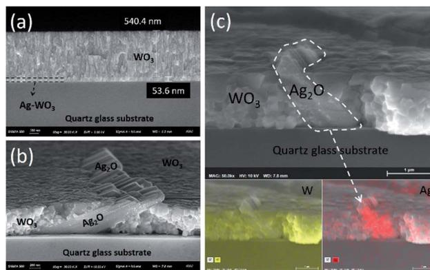
Fig. 4 FESEM images of  $\text{WO}_3/\text{Ag}-\text{WO}_3$  thin films: (a) cross-section of the as-deposited films, (b) cross-section of the annealed films at 923 K, (c) cross-section of backscattering image and EDS elemental mapping of W and Ag corresponding to the annealed films at 923 K.
