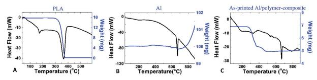
Fig. 2 (A), (B) and (C) DSC and TGA of PLA, Al, and the as-printed Al/polymer-composite, respectively. The phase transformation of the as-printed Al/polymer-composite was the same as those of PLA and Al in combination.
