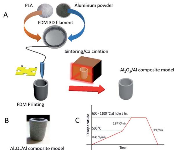
Fig. 1 (A) Schematic of the fabrication of the Al<sub>2</sub>O<sub>3</sub>/Al composite refractory. (B) The Al<sub>2</sub>O<sub>3</sub>/Al composite refractory after sintering and calcination. (C) Temperature profile during the sintering and calcination process.
