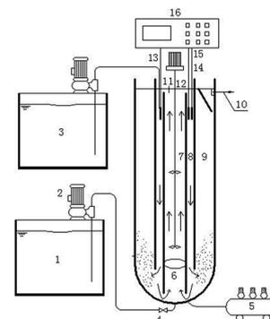
Fig. 1 Schematic diagram of experimental setup: (1)  $\text{NH}_4\text{Cl}$  feeding container, (2) feeding pump, (3)  $\text{Na}_2\text{CO}_3$  feeding container, (4) valve, (5) air pump, (6) annular tube aerator, (7) agitation zone, (8) diversion zone, (9) sedimentation zone, (10) outlet, (11) sampling port, (12) stirrer, (13) pH probe, (14) temperature probe, (15) DO probe, and (16) operation interface.
