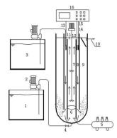
Fig. 1 Schematic diagram of experimental setup: (1)  $NH_4Cl$  feeding container, (2) feeding pump, (3)  $Na_2CO_3$  feeding container, (4) valve, (5) air pump, (6) annular tube aerator, (7) agitation zone, (8) diversion zone, (9) sedimentation zone, (10) outlet, (11) sampling port, (12) stirrer, (13) pH probe, (14) temperature probe, (15) DO probe, and (16) operation interface
