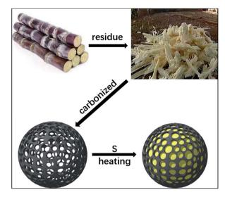
Fig. 1 The preparation process of S/BC composite.
