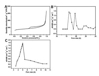
Fig. 2 N<sub>2</sub> adsorption/desorption isotherms of S/BC (A); pore size distribution plots calculated by H-K (B) and DFT of S/BC (C).
