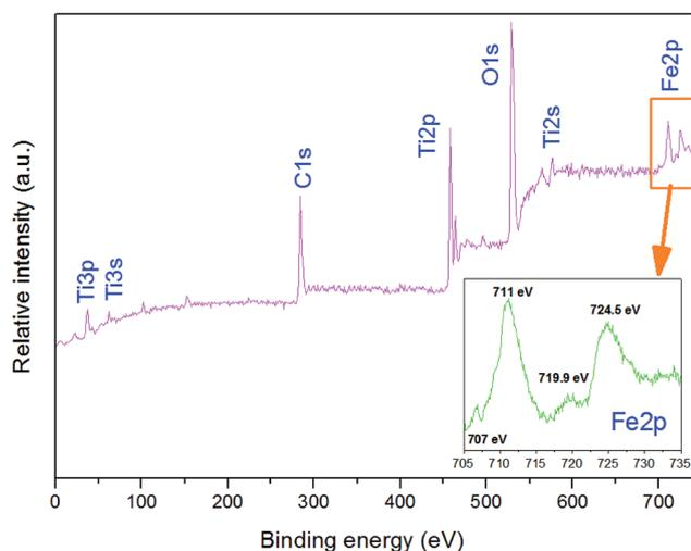
Fig. 5 XPS survey spectra of the as-synthesized 3D-TiO<sub>2</sub>/nano-Fe<sup>0</sup> photocatalysts.
