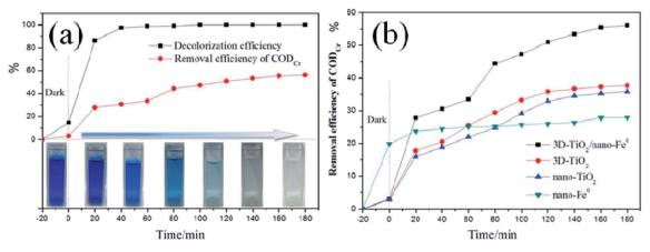
Fig. 9 (a), Comparison of decolorization rate and  $COD_{Cr}$  in photocatalytic process. (b),  $COD_{Cr}$  removal rate under the different samples.
