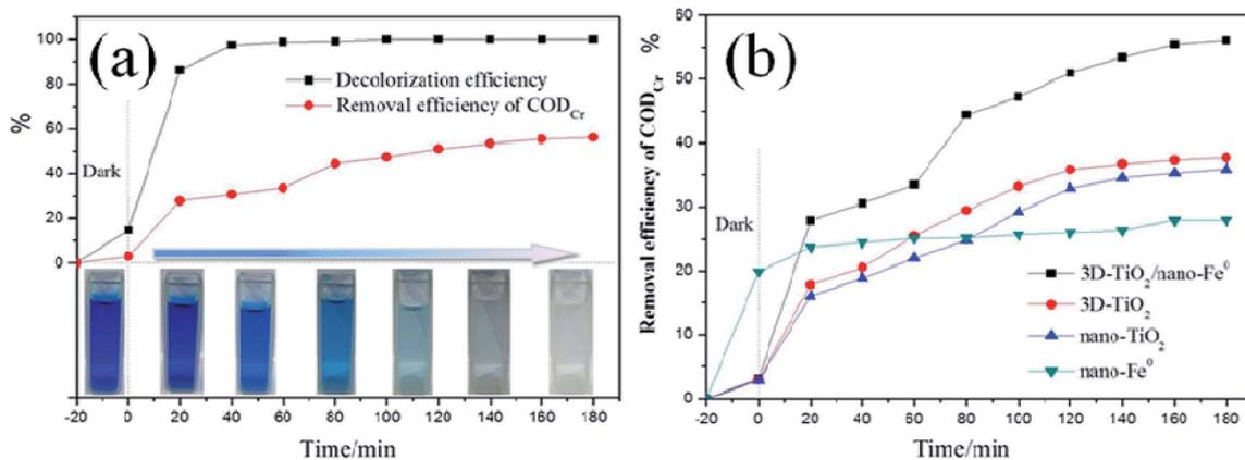
Fig. 9 (a), Comparison of decolorization rate and COD<sub>Cr</sub> in photocatalytic process. (b), COD<sub>Cr</sub> removal rate under the different samples.
