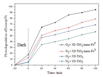
Fig. 7 Comparion on photocatalytic degradation activity of samples under the different concentration of dissolved oxygen.
