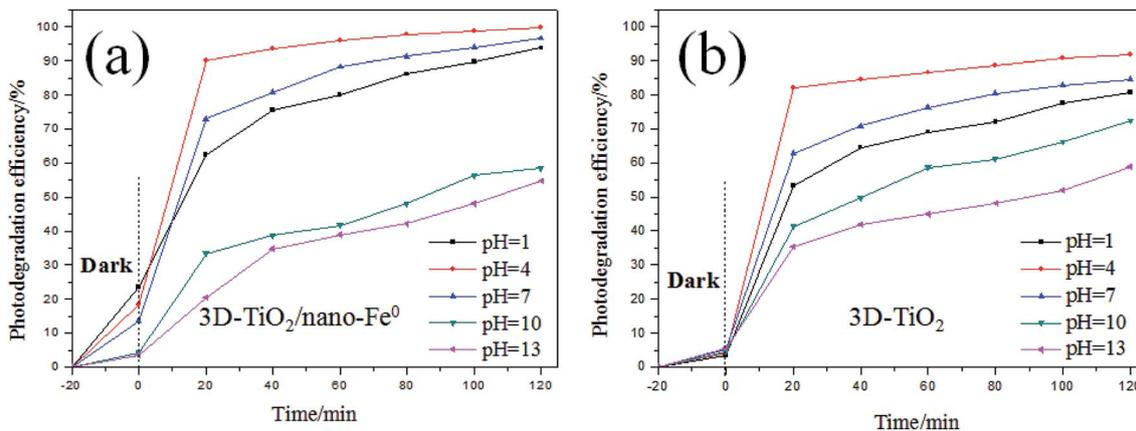
Fig. 6 Comparison on photocatalytic degradation activity of samples under different pH. (a) 3D-TiO<sub>2</sub>/nano-Fe<sup>0</sup>; (b) 3D-TiO<sub>2</sub>.
