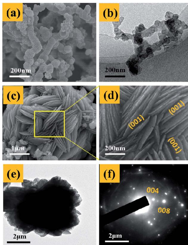
Fig. 3 Microstructure and morphology of samples. (a) and (b), SEM and TEM images of typical nano-Fe<sup>0</sup> particles. (c) and (d), SEM images of typical 3D-TiO<sub>2</sub>. (e), TEM images of 3D-TiO<sub>2</sub>. The corresponding selected-area electron diffraction (SAED) patterns was shown in (f).
