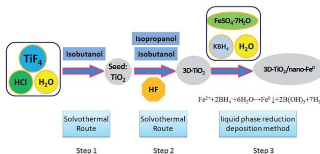
Scheme 1 Synthesis route of 3D laminated structure anatase TiO<sub>2</sub>/nano-Fe<sup>0</sup> photocatalysts (3D-TiO<sub>2</sub>/nano-Fe<sup>0</sup>).
