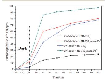
Fig. 8 Comparion on photocatalytic degradation activity of samples under UV light and under visible light.
