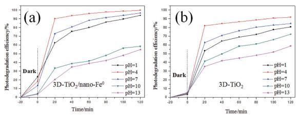
Fig. 6 Comparion on photocatalytic degradation activity of samples under different pH. (a) 3D-TiO<sub>2</sub>/nano-Fe<sup>0</sup>; (b) 3D-TiO<sub>2</sub>.
