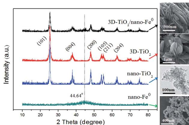
Fig. 1 XRD patterns of nano-Fe<sup>0</sup>; nano-TiO<sub>2</sub>; 3D-TiO<sub>2</sub> and 3D-TiO<sub>2</sub>/nano-Fe<sup>0</sup>.
