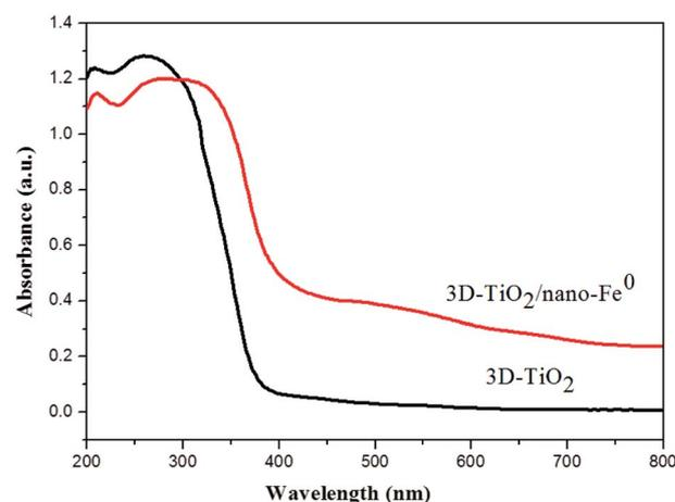
Fig. 2 UV-vis DRS of the 3D-TiO<sub>2</sub> and 3D-TiO<sub>2</sub>/nano-Fe<sup>0</sup> photocatalyst.
