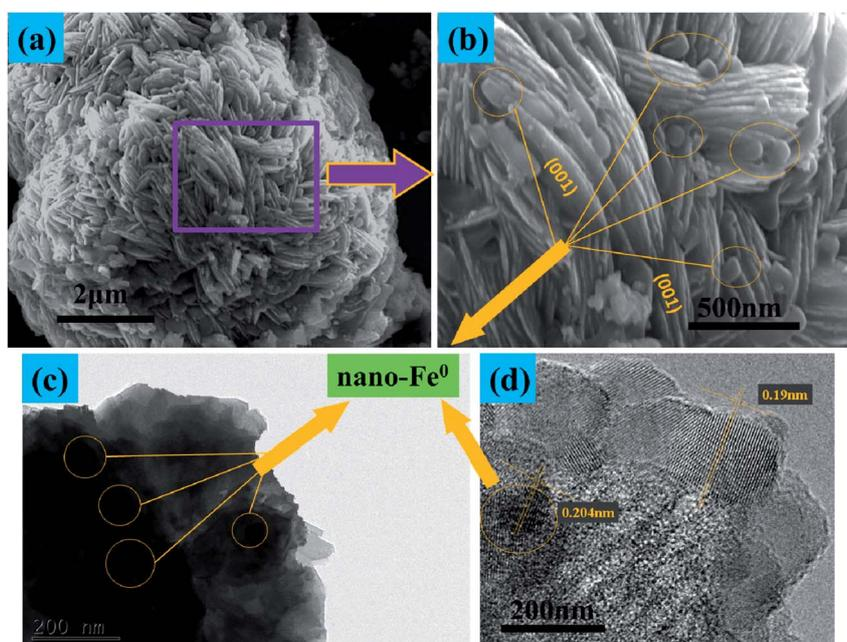
Fig. 4 (a) and (b), SEM images of typical 3D-TiO<sub>2</sub>/nano-Fe<sup>0</sup> photocatalysts. (c) and (d), TEM and HRTEM images of 3D-TiO<sub>2</sub>/nano-Fe<sup>0</sup> photocatalysts.
