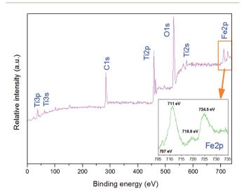
Fig. 5 XPS survey spectra of the as-synthesized  $3D\text{-TiO}_2/\text{nano-Fe}^0$  photocatalysts.
