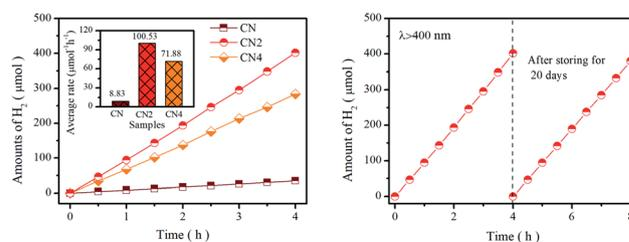
Fig. 6 (a) Amount of  $H_2$  generation of CN, CN2, and CN4 under the irradiation of visible light ( $\lambda > 400 \text{ nm}$ ), (b) comparison of the  $H_2$  generation rate between the first cycle and after storing for 20 days for CN2.
