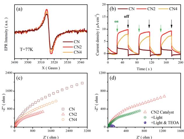
Fig. 5 (a) EPR spectra, and (b) transient photocurrent response, and (c) Nyquist plots of CN, CN2 and CN4. (d) Nyquist plots of CN2 at different condition.
