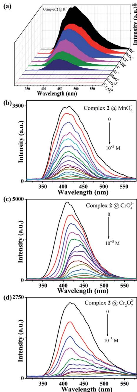
Fig. 3 (a) Fluorescence spectra of 2 immersed into aqueous solution containing various anions; (b) fluorescence spectra of quantitatively titrating the  $\text{MnO}_4^{2-}$ , (c)  $\text{CrO}_4^{2-}$  and (d)  $\text{Cr}_2\text{O}_7^{2-}$  anion aqueous solution into the suspension of complex 2 (concentration range is from 0 to  $10^{-3}$  M).
