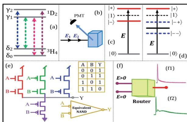
Fig. 1 (a) Energy level of Pr<sup>3+</sup>:YPO<sub>4</sub>. (b) Experimental setup. (c) Single dressed energy level. (d) Double dressed energy level. (e) The schematic diagram of the MOSFET logic "NAND" gate, where (A, B) and Y is the input and output of proposed equivalent logic NAND gate, respectively. (f) The schematic diagram of the multi-channel router.
