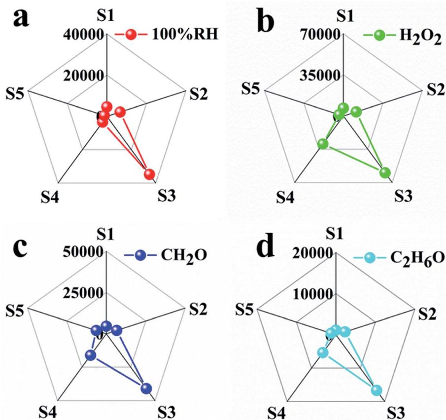
Fig. 6 Characteristic fingerprints deduced by combining kinetic and thermodynamic parameters from sensing data of (a) 100% RH, (b) saturated vapors of  $\text{H}_2\text{O}_2$  at room temperature, (c)  $\text{CH}_2\text{O}$ , (d)  $\text{C}_2\text{H}_6\text{O}$ .
