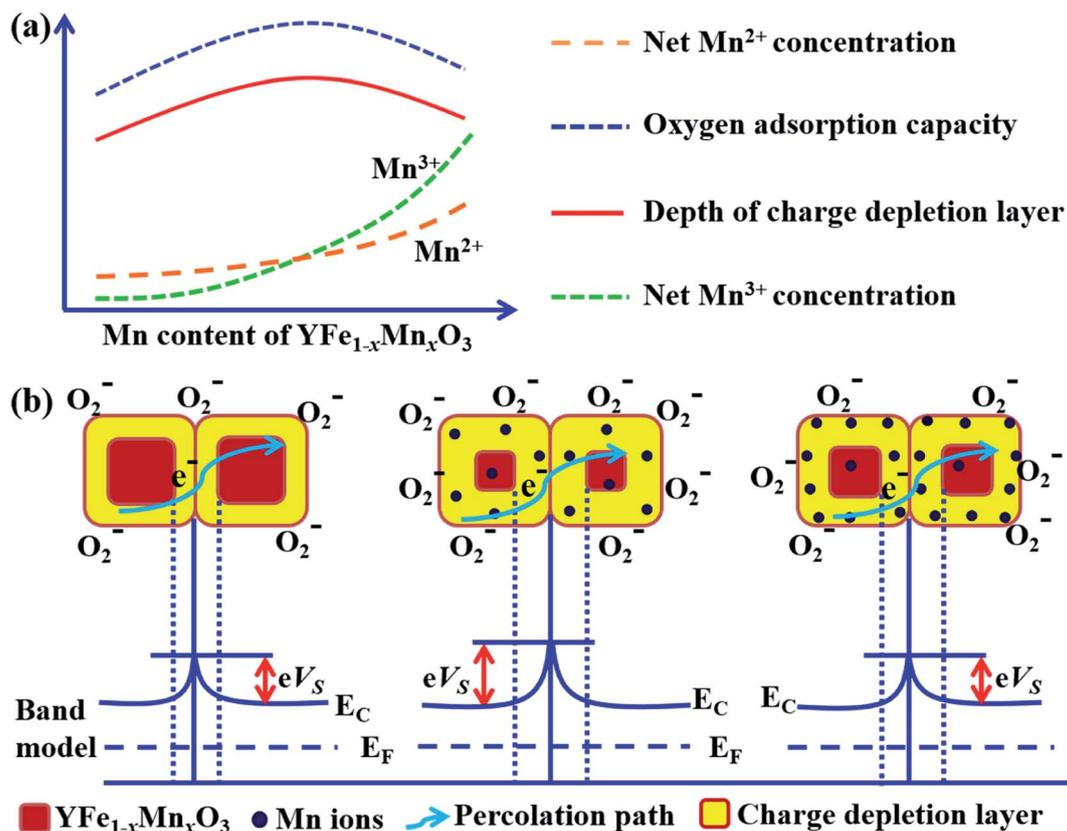
Fig. 9 (a) The variation of net  $Mn^{2+}$  and  $Mn^{3+}$  concentrations with the increase of Mn doping, and the influence on oxygen adsorption capacity and the charge depletion layer, (b) structural and band models showing the role of Mn doping of the charge depletion layer of  $YFe_{1-x}Mn_xO_3$ .
