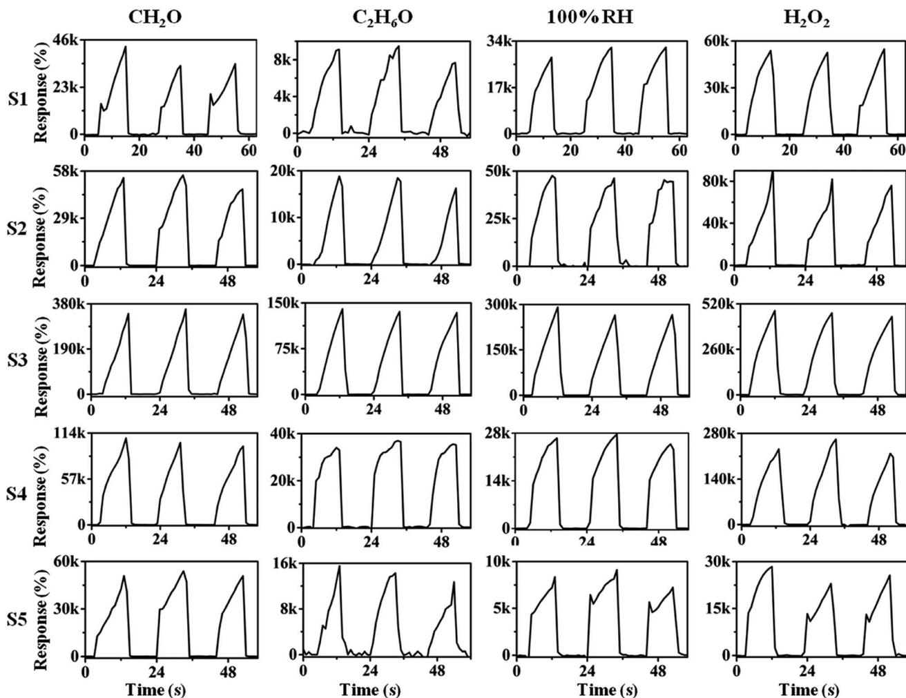
Fig. 4 Sensing curves of different sensors based on  $\text{YFe}_{1-x}\text{Mn}_x\text{O}_3$  to 1000 ppm of  $\text{CH}_2\text{O}$ ,  $\text{C}_2\text{H}_6\text{O}$ ,  $\text{H}_2\text{O}_2$  and 100% RH at room temperature.
