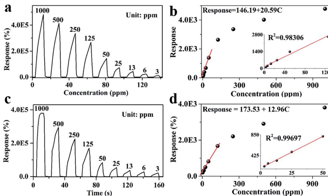
Fig. 8 Relation between responses of S3 and vapor concentrations at RT of (a)  $\text{H}_2\text{O}_2$ , (c)  $\text{CH}_2\text{O}$ ; the fitting plots of response vs. concentration of (b)  $\text{H}_2\text{O}_2$ , (d)  $\text{CH}_2\text{O}$ .
