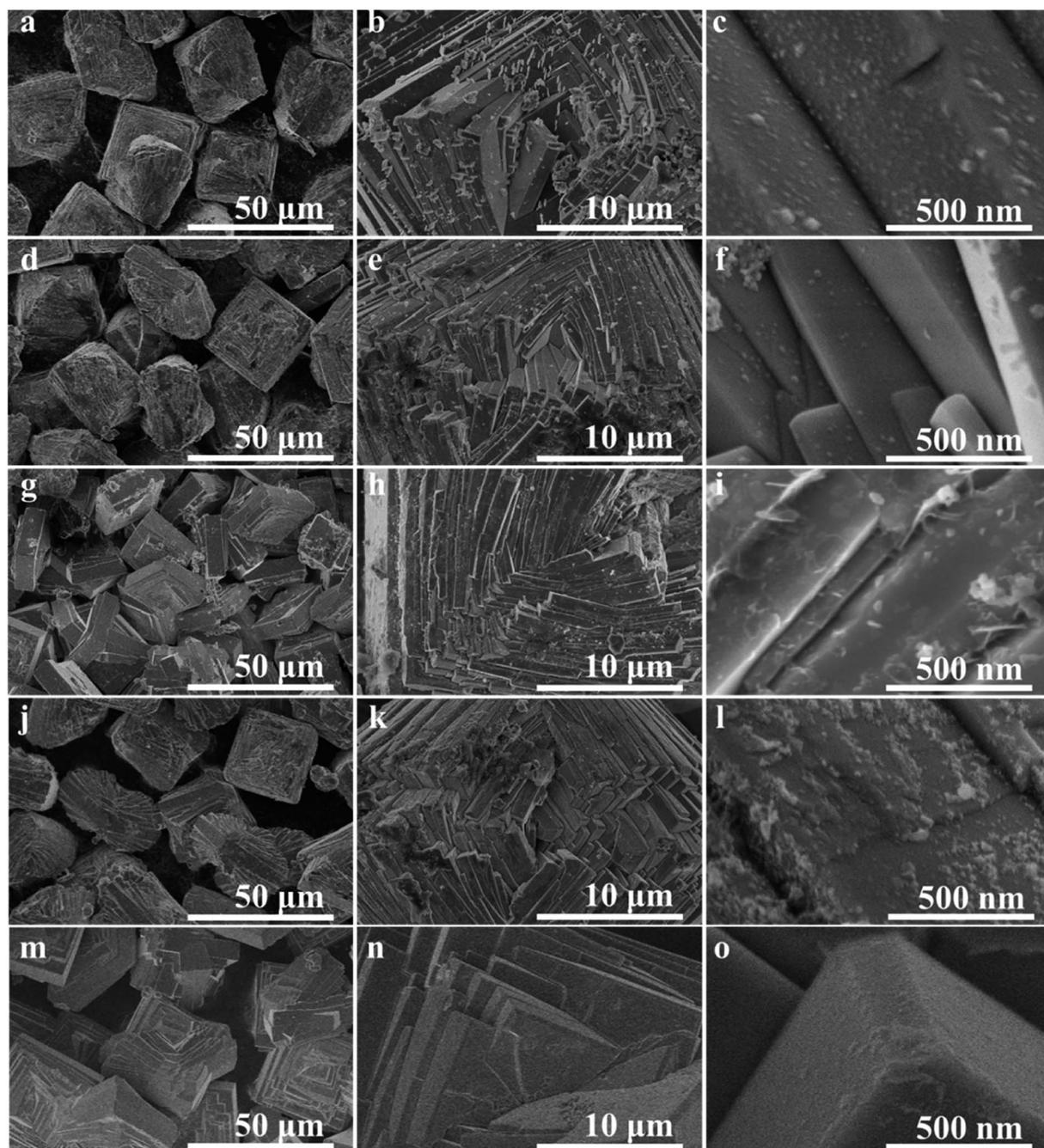
Fig. 1 SEM images of five samples (a–c)  $\text{YFeO}_3$ , (d–f)  $\text{YFe}_{0.975}\text{Mn}_{0.025}\text{O}_3$ , (g–i)  $\text{YFe}_{0.95}\text{Mn}_{0.05}\text{O}_3$ , (j–l)  $\text{YFe}_{0.925}\text{Mn}_{0.075}\text{O}_3$ , and (m–o)  $\text{YFe}_{0.9}\text{Mn}_{0.1}\text{O}_3$ .
