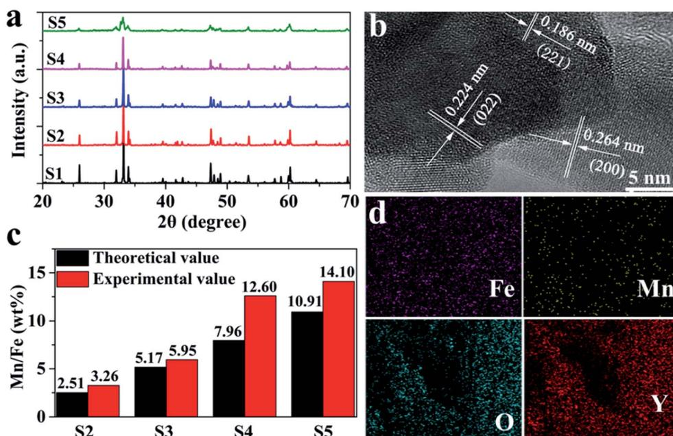
Fig. 2 (a) XRD patterns, (b) HRTEM images, (c) content of Mn element in  $\text{YFe}_{1-x}\text{Mn}_x\text{O}_3$  according to EDS test, and (d) EDS mappings of the samples.
