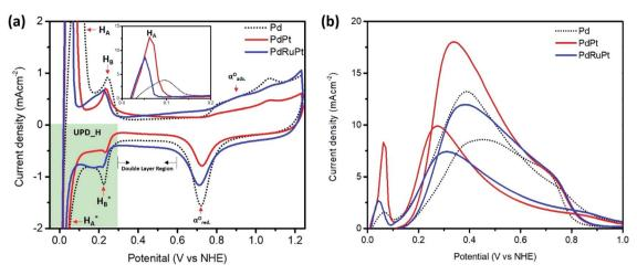
Fig. 5 (a) The CV curves of experimental NCs recorded in  $N_2$  saturated 0.5 M  $H_2SO_4$  electrolyte solution and (b) the LSV patterns of Pd, PdPt, and PdRuPt NCs recorded in  $N_2$  saturated 0.5 M  $H_2SO_4$  and 0.5 M HCOOH electrolyte solution.
