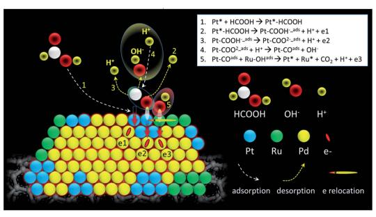
Scheme 1 Reaction coordinates of formic acid oxidation on PdRuPt surface. The first four steps adopt to all experimental samples. The 5th step, which is the key reaction step, only adopt in the presence of Ru atoms on catalyst surface.
