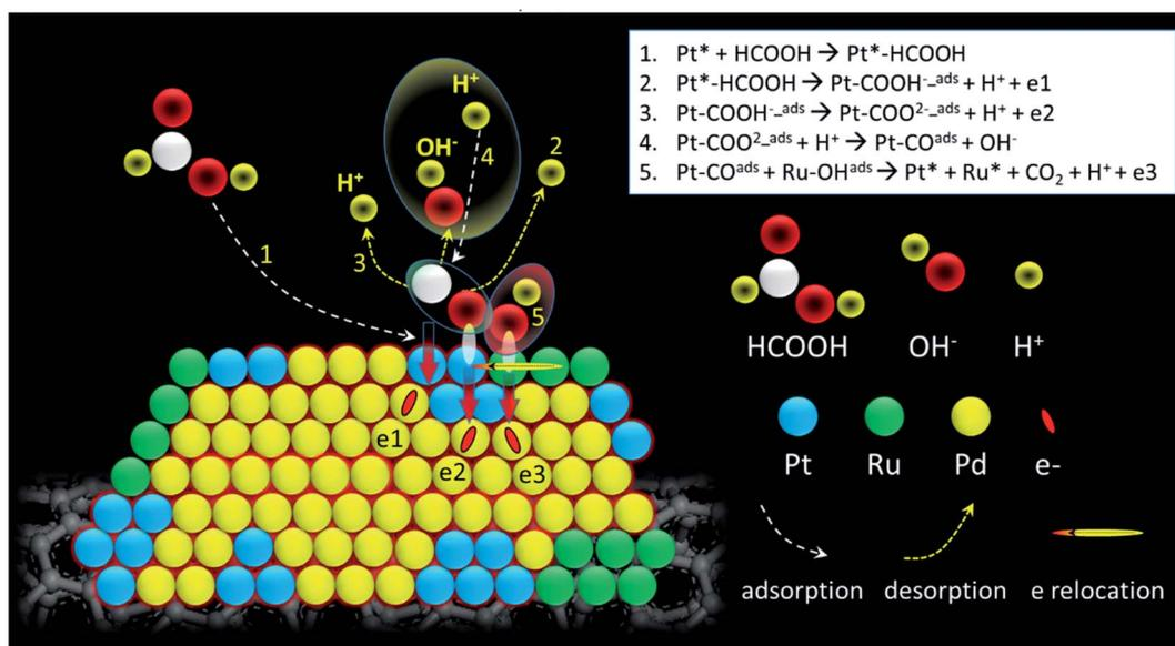
**Scheme 1** Reaction coordinates of formic acid oxidation on PdRuPt surface. The first four steps adopt to all experimental samples. The 5th step, which is the key reaction step, only adopt in the presence of Ru atoms on catalyst surface.
