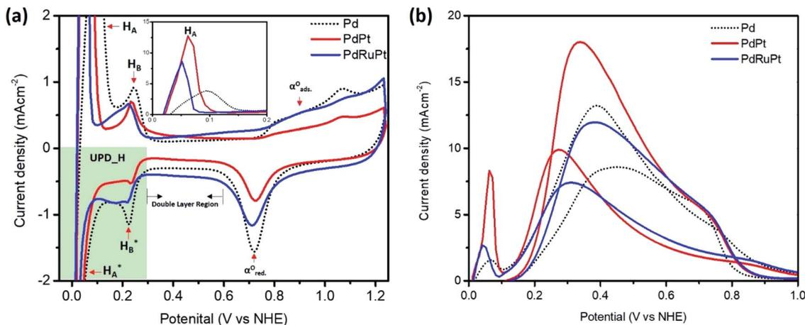
Fig. 5 (a) The CV curves of experimental NCs recorded in  $N_2$  saturated 0.5 M  $H_2SO_4$  electrolyte solution and (b) the LSV patterns of Pd, PdPt, and PdRuPt NCs recorded in  $N_2$  saturated 0.5 M  $H_2SO_4$  and 0.5 M  $HCOOH$  electrolyte solution.
