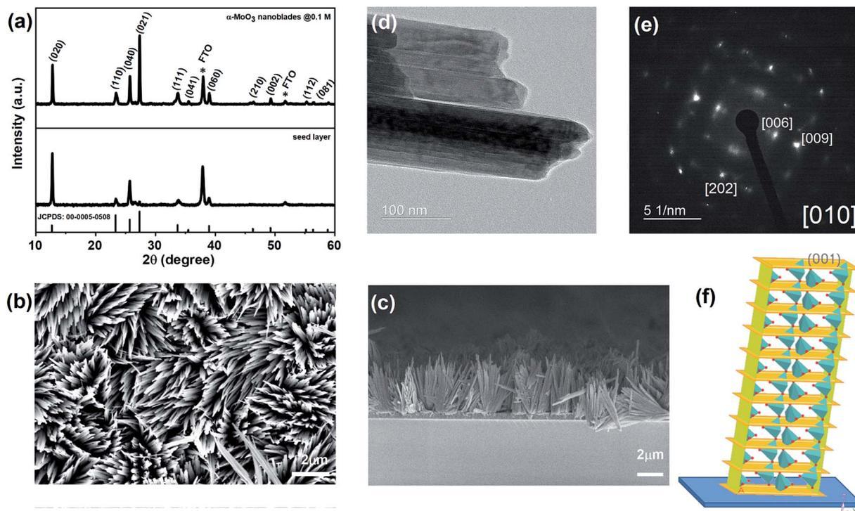
Fig. 3 (a) XRD spectra of the annealed seed layer and vertically aligned  $\alpha$ - $\text{MoO}_3$  nano-blades on FTO substrates, (b and c) FE-SEM images of vertically aligned  $\alpha$ - $\text{MoO}_3$  nano-blades, (d and e) HRTEM-SAED of  $\alpha$ - $\text{MoO}_3$  nano-blades, (f) Schematic of  $\text{MoO}_3$ -nano-blades growth planes on the substrate.
