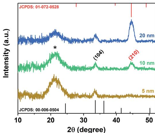
Fig. 2 GIXRD patterns of annealed chromium layer on  $\text{Si}/\text{SiO}_2$  substrates, with corresponding stick patterns of  $\text{Cr}_2\text{O}_3$  (black) and  $\text{Cr}_3\text{O}$  (red), respectively. The star indicates the amorphous  $\text{SiO}_2$  peak.
