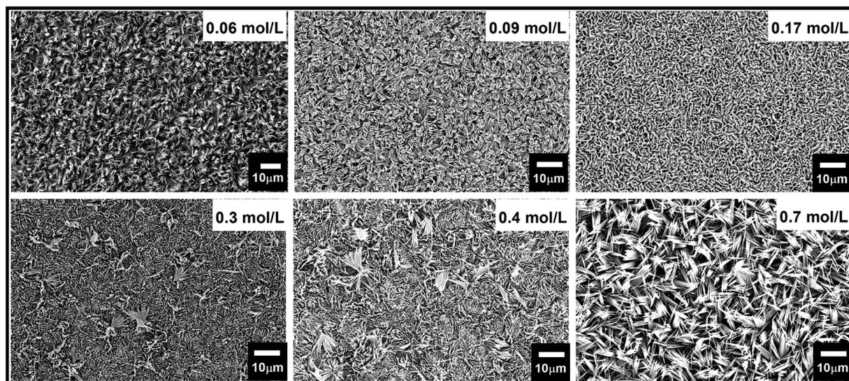
Fig. 5 FE-SEM micrographs of vertically aligned  $\alpha$ -MoO<sub>3</sub> nano-blades prepared by varying the acid molar concentration at a growth temperature of 180 °C on the seeded substrate of 10/100 nm of Cr/MoO<sub>3</sub>.
