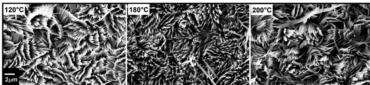
Fig. 7 FE-SEM micrographs of vertically aligned  $\alpha$ -MoO<sub>3</sub> nano-blades prepared at different hydrothermal reaction's temperatures using acid molar concentration of 0.3 mol L<sup>-1</sup> and seed layer of 10/100 nm of Cr/MoO<sub>3</sub>.
