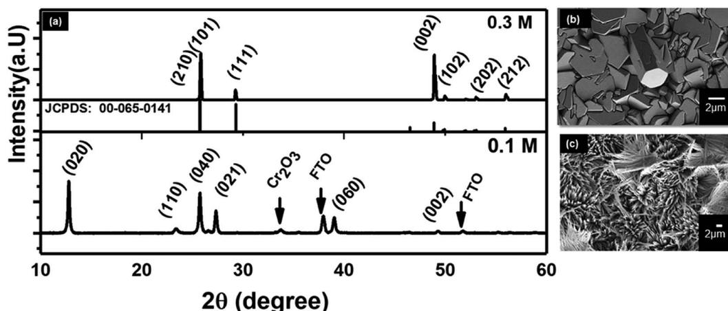
Fig. 6 XRD patterns of MoO<sub>3</sub> nanostructures at a different molar concentration at 180 °C using seed layer of Cr/MoO<sub>3</sub> of 10/100 nm (a) 0.1 M and 0.3 M. FE-SEM images of MoO<sub>3</sub> nanostructures at a different molar concentration (b) 0.1 M and (c) 0.3 M.
