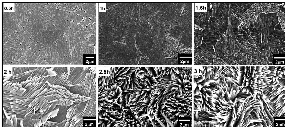
Fig. 4 FE-SEM micrographs show the growth of vertically aligned  $\alpha$ - $\text{MoO}_3$  on FTO at different times during the hydrothermal reaction using  $0.3 \text{ mol L}^{-1}$  acid concentration and reaction temperature of  $180^\circ\text{C}$ .
