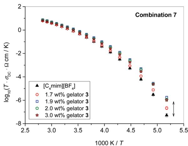
Fig. 2 Ionic conductivity as a function of reciprocal temperature for neat  $[C_4mim][BF_4]$  and ionogels from combination 7 with various concentrations of gelator 3. The error bars are at most of the order of the symbol size.
