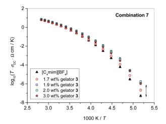
Fig. 2 Ionic conductivity as a function of reciprocal temperature for neat  $[C_4 \text{mim}][BF_4]$  and ionogels from combination 7 with various concentrations of gelator 3. The error bars are at most of the order of the symbol size.
