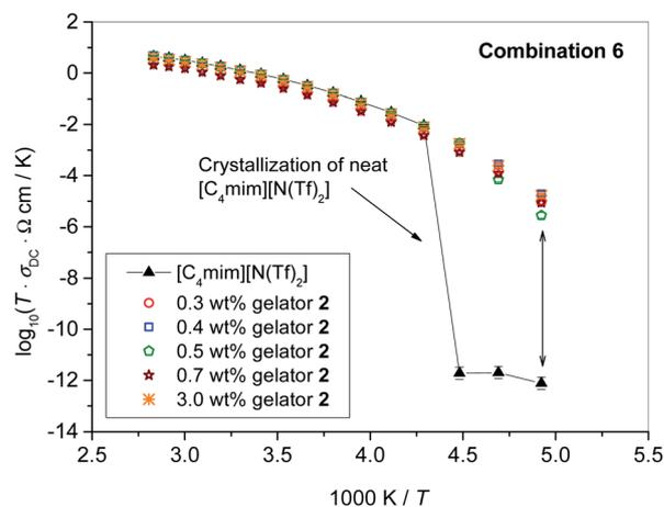
Fig. 3 Ionic conductivity as a function of reciprocal temperature for neat  $[C_4mim][N(Tf)_2]$  and ionogels of combination 6 with various concentrations of gelator 2. The line connecting the data for  $[C_4mim][N(Tf)_2]$  is a guide to the eye. The error bars are at most of the order of the symbol size.
