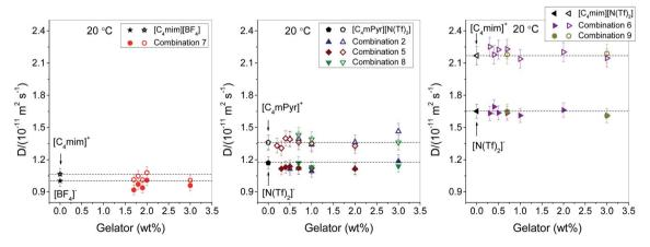
Fig. 4 Diffusion coefficients of cations and anions at 20 °C for the neat ionic liquids and ionogels of various combinations as a function of gelator concentration. Open symbols: cation; full symbols: anion.
