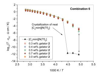
Fig. 3 Ionic conductivity as a function of reciprocal temperature for neat  $[C_4 \text{mim}][N(Tf)_2]$  and ionogels of combination 6 with various concentrations of gelator 2. The line connecting the data for  $[C_4 \text{mim}][N(Tf)_2]$  is a guide to the eye. The error bars are at most of the order of the symbol size.
