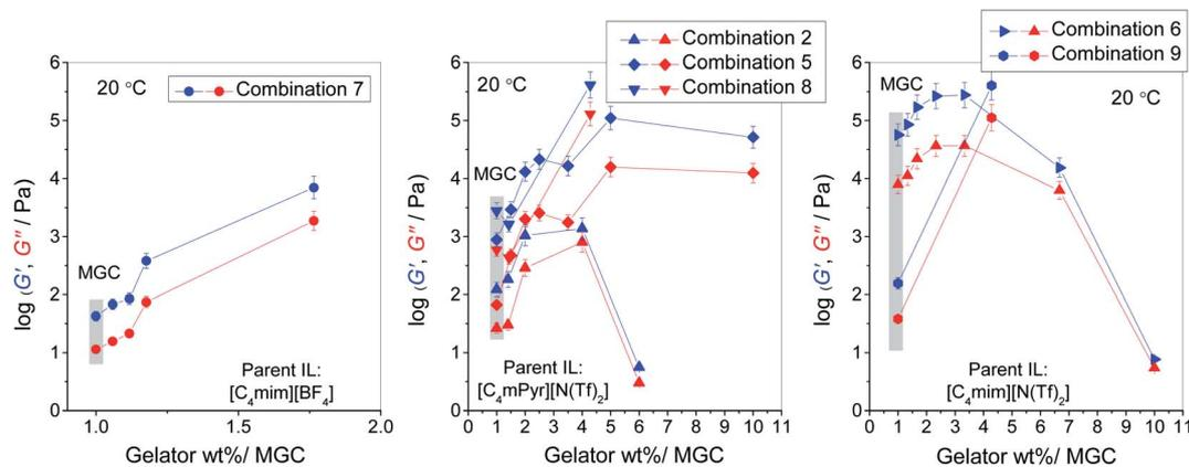
Fig. 6 Storage ( $G'$ ) and loss ( $G''$ ) modulus at 20 °C of various ionogels as a function of gelator concentration normalized by the MGC. Blue symbols:  $G'$ , red symbols:  $G''$ . Lines are guides to the eye.
