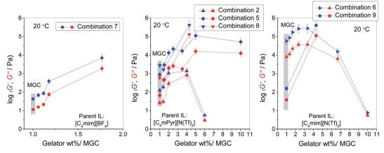
Fig. 6 Storage (G') and loss (G'') modulus at 20 °C of various ionogels as a function of gelator concentration normalized by the MGC. Blue symbols: G', red symbols: G''. Lines are guides to the eye.
