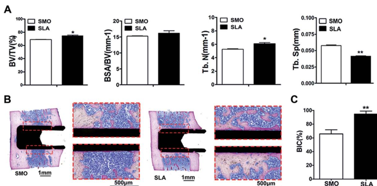
Fig. 3 hBMSC adhesion, proliferation, and osteogenic differentiation on SLA and SMO surfaces *in vivo*. (A) BV/TV, BSA/BV, Tb.N, and Tb.Sp. (B) Histological sections were stained with methylene blue-basic fuchsin. The red frame represents the peri-implant segments of interest. (C) The BIOQUANT OSTEO Bone Biology Research System was used for automatically compute BIC. Data are presented as the mean  $\pm$  s.d. ( $n = 6$ ). \* $p < 0.05$ ; \*\* $p < 0.01$ .
