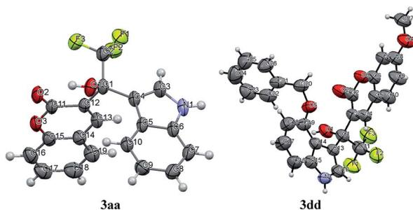
Fig. 1 X-ray structures of products **3aa** and **3dd**.
