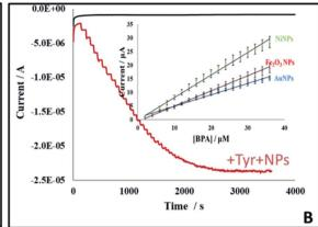
Fig. 5 Enzyme-based detection of BPA by NP amplification using screen printed electrodes modified with Au, Ni or  $Fe_2O_3$  NPs: sensor design (A) and amperometric response with comparative calibration curve (B) showing differential responses to the three types of NPs of which Ni NPs showed the highest sensitivity (schematic summarizing detection platform and results reported in ref. 33).
