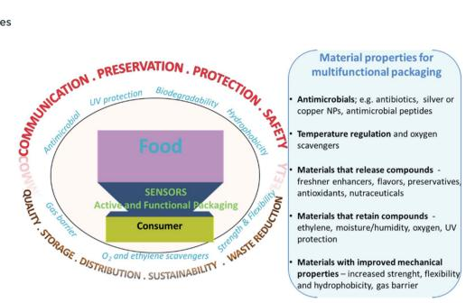
Fig. 12 Illustration of the main properties and applications of active and functional sensors and materials for packaging applications.
