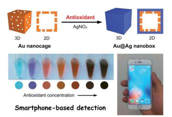
Fig. 3 The sensing principle of antioxidant based on the morphological change of An nanocage upon the reduction of  $AgNO_3$  producing Au@Ag nanobox in presence of antioxidants. Adapted from ref. 48 with permission from Royal Society of Chemistry, Copyright 2018
