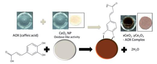
Fig. 4 Reaction mechanism of CeO<sub>2</sub> NPs with antioxidants for the colorimetric detection of antioxidants using caffeic acid as an example. In presence of antioxidants, the color of the NPs change from white/yellowish to dark brown due to surface oxidation and formation of charge transfer complexes. Adapted with modification from ref. 31 and a permission from Royal Society of Chemistry, Copyright 2013.
