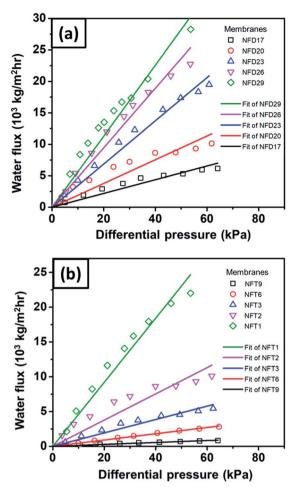
Fig. 11 The water flux vs. differential pressure for nylon 6 nanofibers/cellulose membranes with the variation of (a) nanofiber diameter and (b) nanofibrous membrane thickness.
