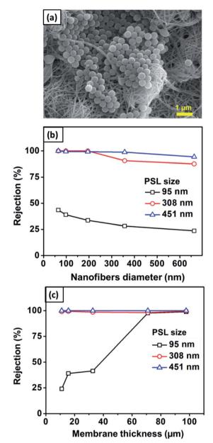
Fig. 12 (a) SEM image of the nanofibrous membrane after filtration. (b) The effect of the nanofiber diameter on the rejection value. (c) The effect of nanofiber thickness on rejection.
