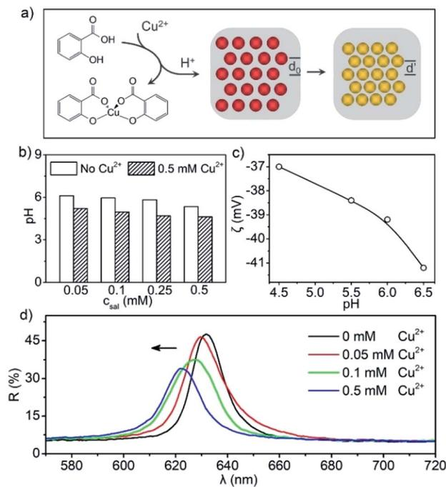
Fig. 2 (a) Schematic illustration to the working mechanism of  $\text{Cu}^{2+}$  sensing by Sal-containing liquid PCs. (b) Change in pH value due to the addition of  $\text{Cu}^{2+}$  and (c) change in particles' zeta potential due to the change in pH value. (d) The reflection of Sal-LPC blueshifts with the increase of  $\text{Cu}^{2+}$  concentration.
