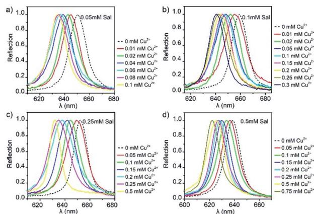
Fig. 4 Optical response of liquid PCs containing (a) 0.05 mM, (b) 0.1 mM, (c) 0.25 mM, and (d) 0.5 mM Sal to the change in  $\text{Cu}^{2+}$  concentration.
