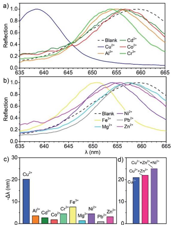
Fig. 7 (a and b) Reflection spectra of the Sal-LPC reagent (blank) and its mixture with solutions of different metal cations. Reflection blueshift due to the addition of (c) single and (d) multiple metal cations to Sal-LPC.
