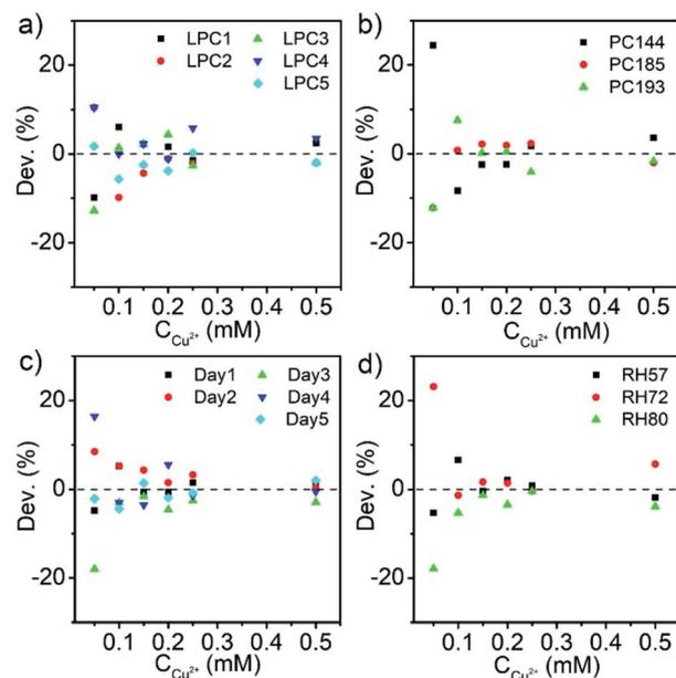
Fig. 8 Deviation of “ $-\Delta\lambda$ ” measured by (a) Sal-LPC prepared in different batches, (b) Sal-LPC prepared by different-sized particles, and the same Sal-LPC (c) in 5 days or (d) at different humidities.
