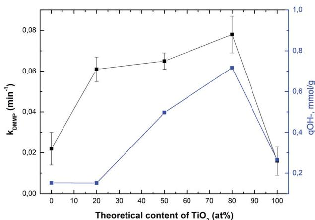
Fig. 4 Correlation between degradation rate constant of DMMP ( $k$ ,  $\text{min}^{-1}$ ) and the theoretical content of  $\text{TiO}_2$ , and the correlation between the amount of hydroxyl groups ( $q\text{-OH}$ ,  $\text{mmol g}^{-1}$ ) and the theoretical content of  $\text{TiO}_2$ .
