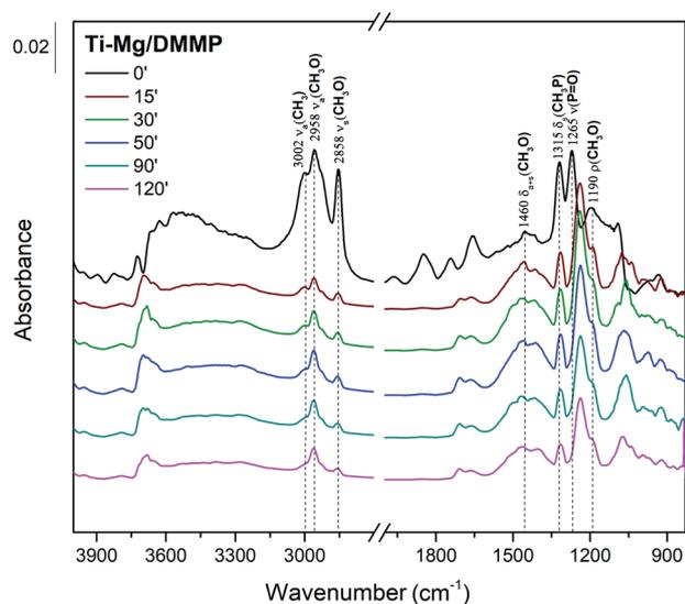
Fig. 6 Time-resolved DRIFTS spectra of DMMP adsorption on the Ti050Mg050 catalyst.
