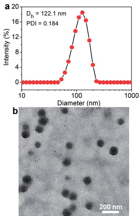
Fig. 4 (a) DLS curve of Ir-C-MMB nanoparticles in water showing the diameter distribution, the polydispersity index (PDI = 0.184), and the average size ( $D_h = 122.1$  nm) of the nanoparticles. (b) TEM image of Ir-C-MMB nanoparticles. Scale bars: 200 nm.
