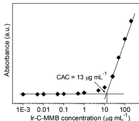
Fig. 3 Relationship between absorbance and the concentration of Ir-C-MMB in aqueous solution ( $\lambda = 313 \text{ nm}$ ,  $25 \text{ }^\circ\text{C}$ ). The CAC value of Ir-C-MMB is about  $13 \mu\text{g mL}^{-1}$ .
