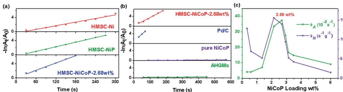
Fig. 4 The corresponding plot of  $-\ln(C/C_0)$  versus reaction time  $t$  (a and b) and NiCoP loading amounts (c). (a) Silicate-nickel alloy composites doped with P and Co, (b) comparison among AHGMs, pure NiCoP, commercial 5 wt% Pd/C and synthesized HMSC–NiCoP–2.68 wt%, (c) the rate constant  $k_A$  and  $k_N$  as a function of NiCoP loading amounts in HMSC–NiCoP.
