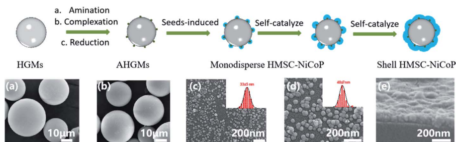
Fig. 3 The schematic illustration formation process of loading NiCoP NPs on HGMs through seeds induced direct assembly fabrication; (a–e) SEM images corresponding with the structural models above in scheme.
