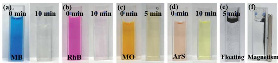
Fig. 7 Photographs of the decolorization of (a) MB, (b) RhB, (c) MO, (d) ArS catalyzed by the HMSC–NiCoP–2.68 wt%; (e) the HMSC–NiCoP–2.68 wt% catalyst floating on the aqueous solution; (f) the separation of HMSC–NiCoP–2.68 wt% catalyst by an magnet.
